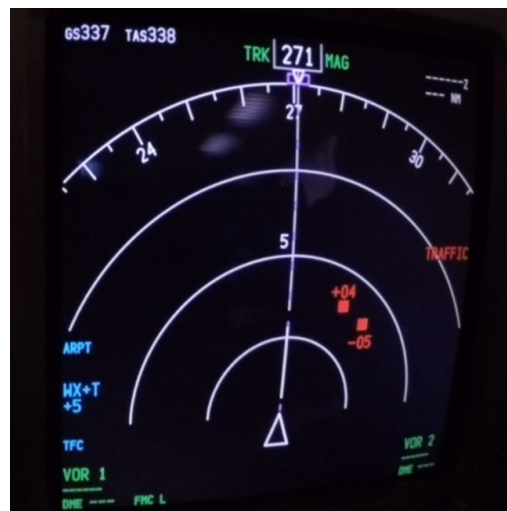
Figure 17: Actual traffic display implementation on Boeing 737-800.
