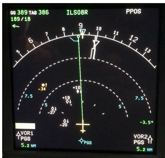
Figure 16: Actual traffic display implementation on Airbus A320.
