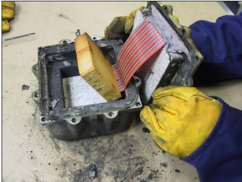
Figure A-8: Polystyrene foam block enclosing the memory board
