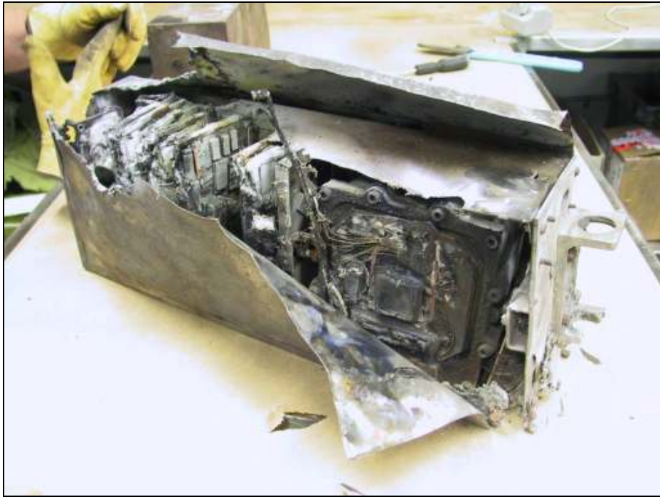
Figure A-6: FDR with the crash-protected memory module visible
