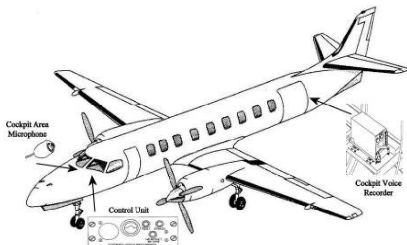
Figure B-7: Location of cockpit voice recorder system components
