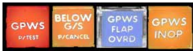
Figure 11: GPWS cockpit annunciators and switches (Image of representative item, not specific item in VH-TFU)
