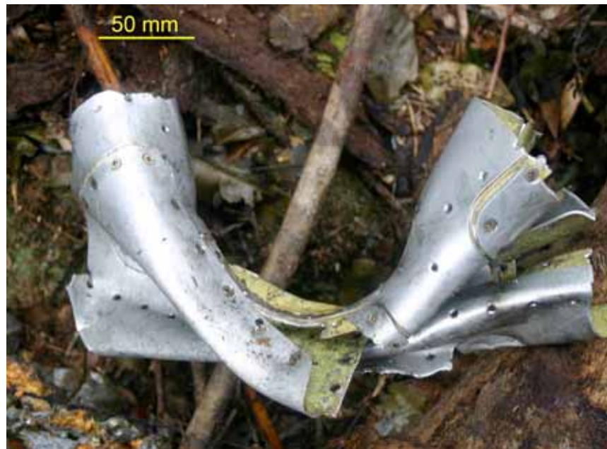
Figure 20: Wing section showing impact damage with a tree trunk or branch
