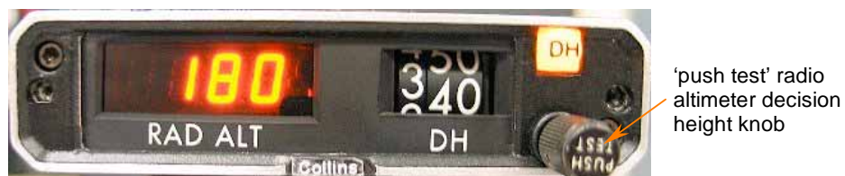
Figure 9: Digital radio altitude indicator (Image of representative item, not specific item in VH-TFU)
