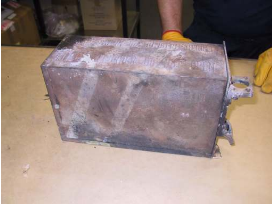
Figure B-1: L-3 Communications Aviation Recorders Fairchild model A100A CVR recovered from VH-TFU
