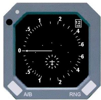
When an intruder aircraft transponder is OFF or SBY, the intruder aircraft is NOT detected by TCAS.
