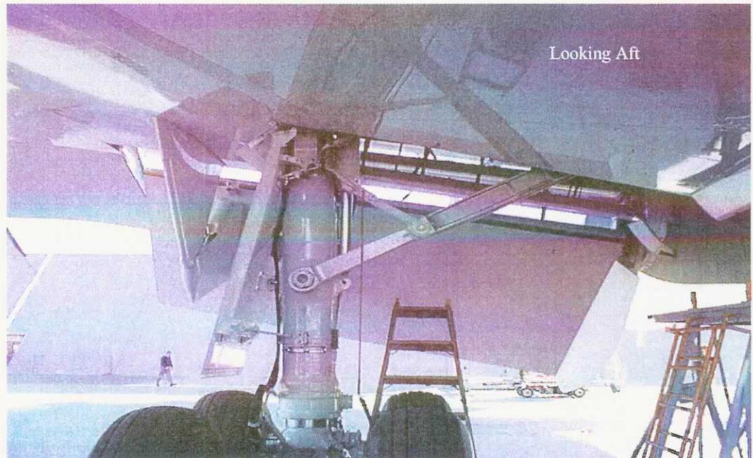
Figure 9. Inboard Flap (Location relative to MLG)
