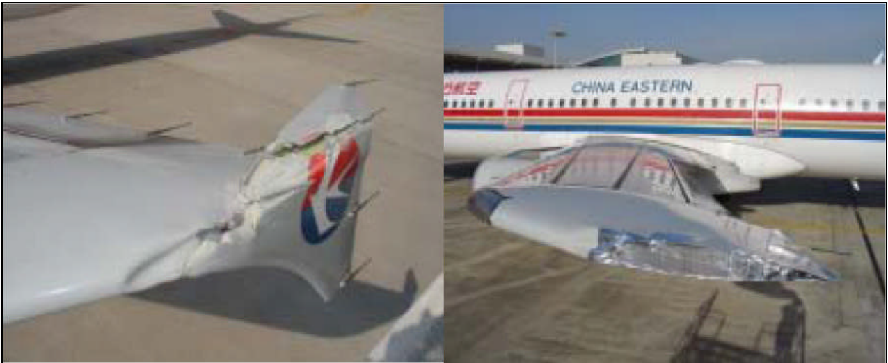
[Picture 1] Picture of damaged left Wing Tip
