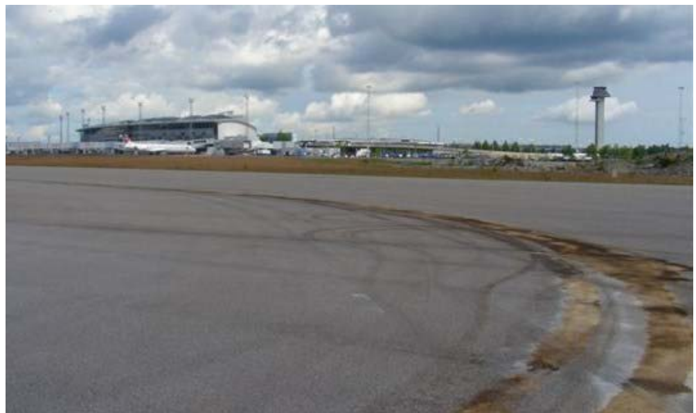
Fig 16. Fuel trail after absorbing agent had been applied.
