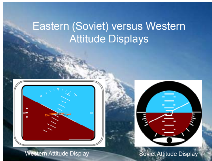
Figure 2---- Western versus Eastern (Soviet Era) Attitude Display Indicators
