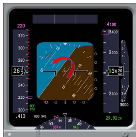
Figure 7— Example ADI / EFIS with a Corrective Arrow for an Excessive Bank Angle Situation
