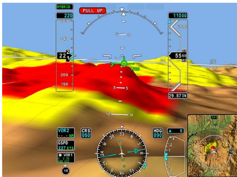
Figure 9-- Synthetic Vision—bringing the outside world inside to the cockpit.
