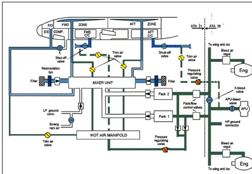
This diagram is a schematic layout of the air circulation system on the Airbus A319
