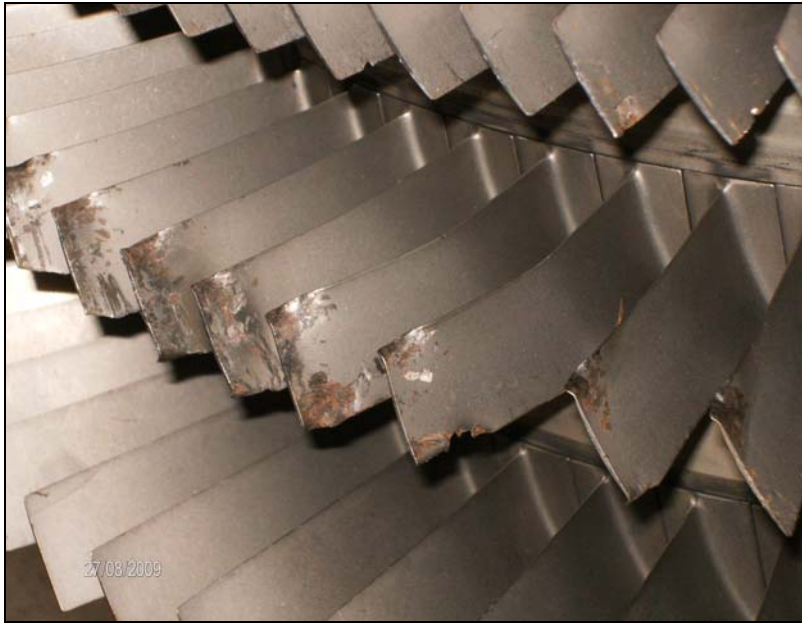
Photo No. 3: Damage to LP Compressor
