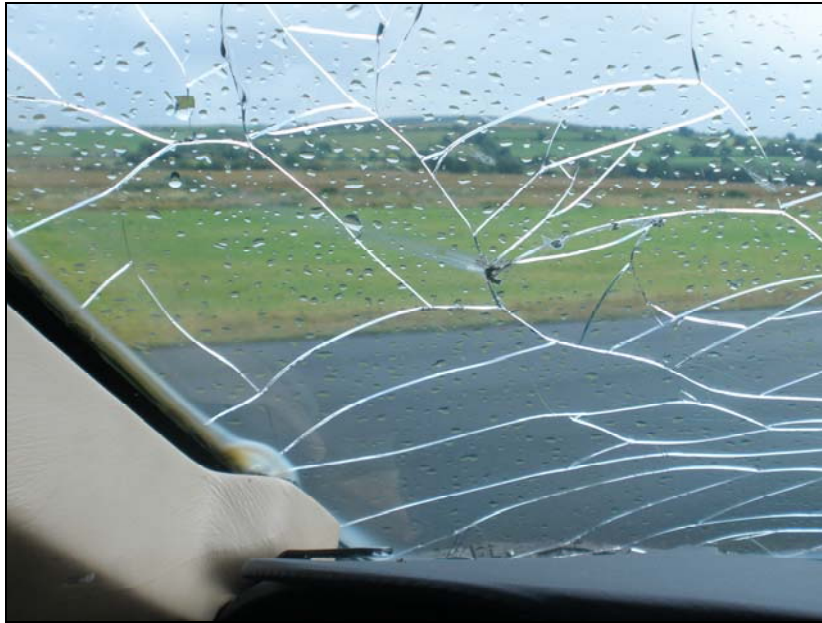
Photo No. 1: Damage to Windshield (Note: The lines are cracks and the dots are raindrops)
