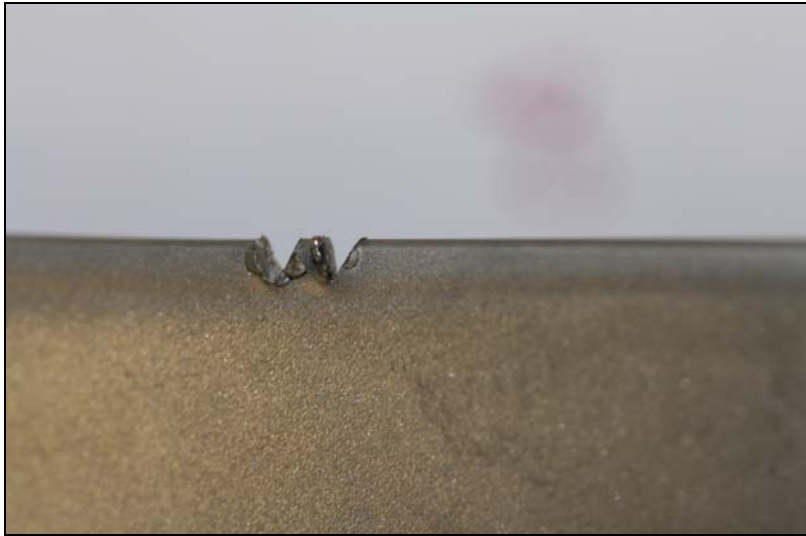
Photo No. 2: Typical Fan Blade Damage (VT-MST)
