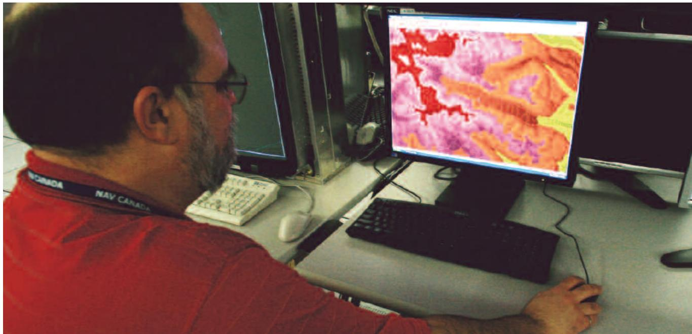
*Colour coded terrain contours used by the NAV CANADA MSAW.*
