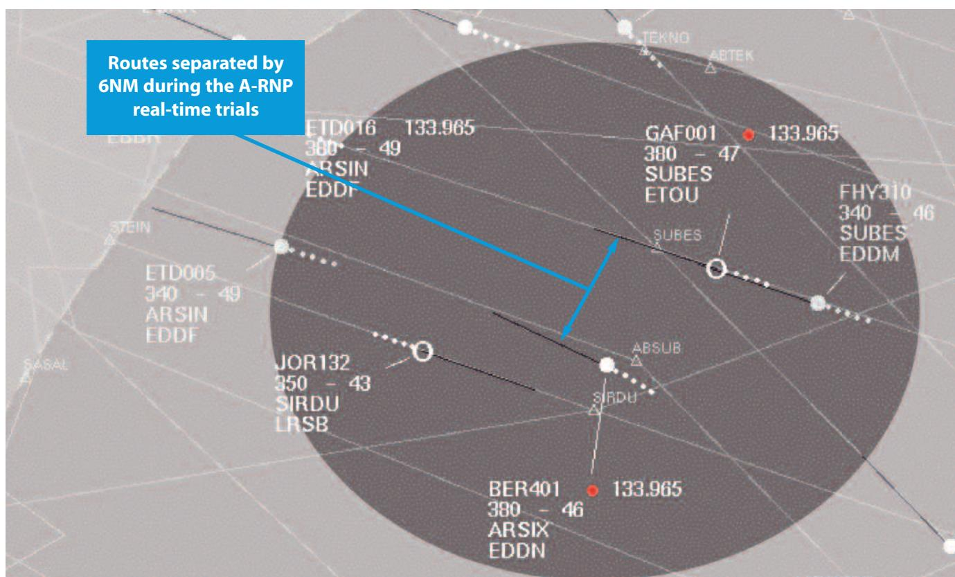
Aircraft operating on parallel routes separated by 6NM during the A-RNP real-time trials
