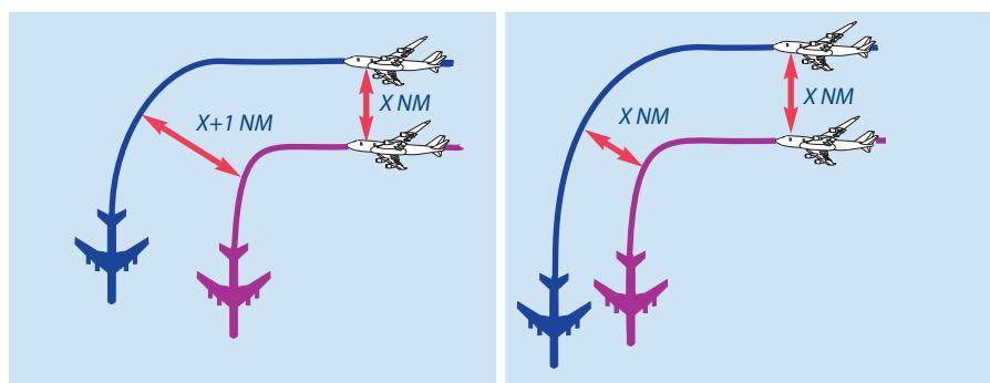
*Simplified images of two aircraft turning on closely spaced routes today (left) and using repeatable turn performance (right).*
