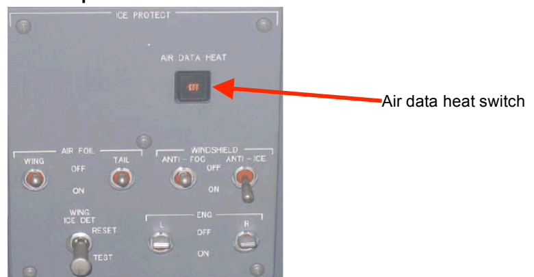
Figure 4: Ice protection control panel - air data heat switch selected OFF
