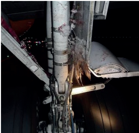
Illustration 3: bird remains found in the left main landing gear
