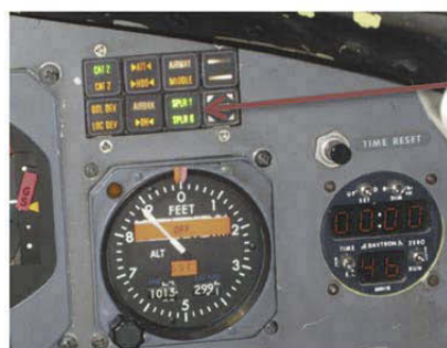
Figure 7: Yellow and green lift spoilers lights.
