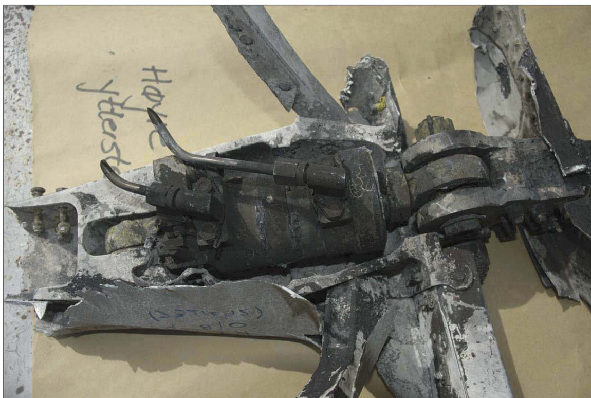
Figure 34: One of the six lift spoiler actuators.
