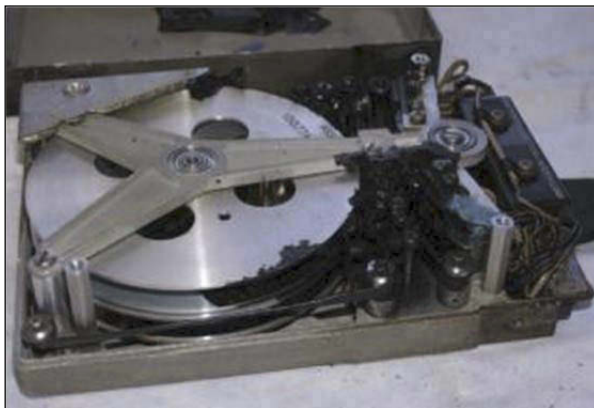
Figure 16: Heat-damaged storage unit in FDR.
