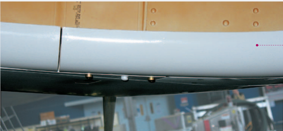
Figure 5: Newly configured exhaust vents designed to reduce drag
