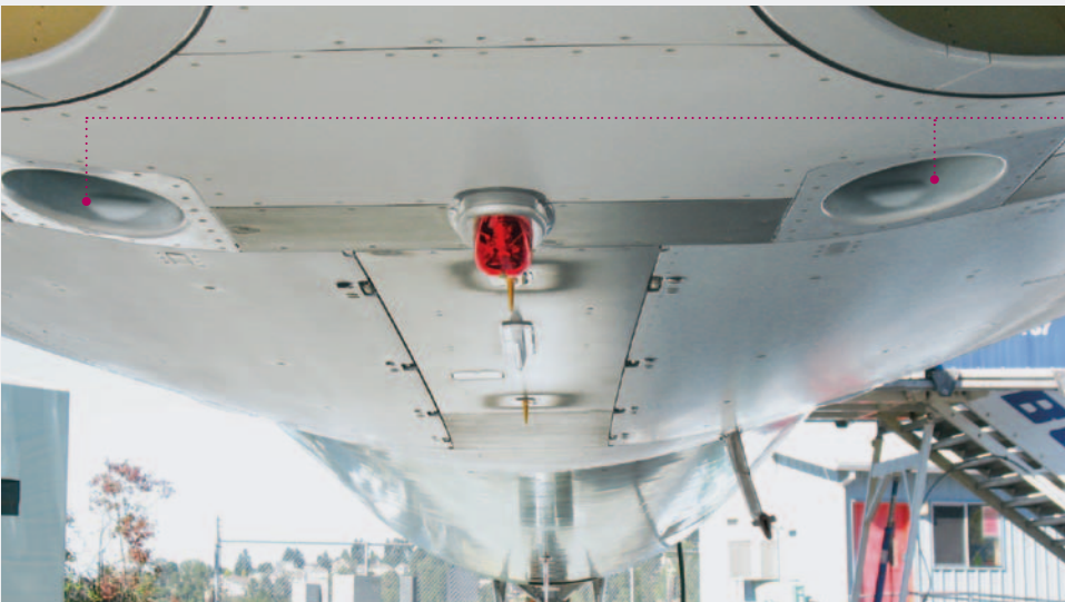
Figure 5: Newly configured exhaust vents designed to reduce drag
