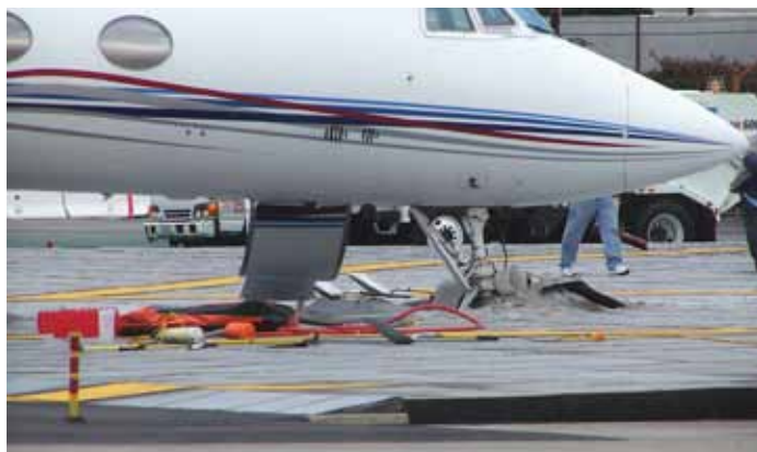
The benefits of EMAS are clearly exhibited in this photo of a plane that was stopped at Burbank Airport.
