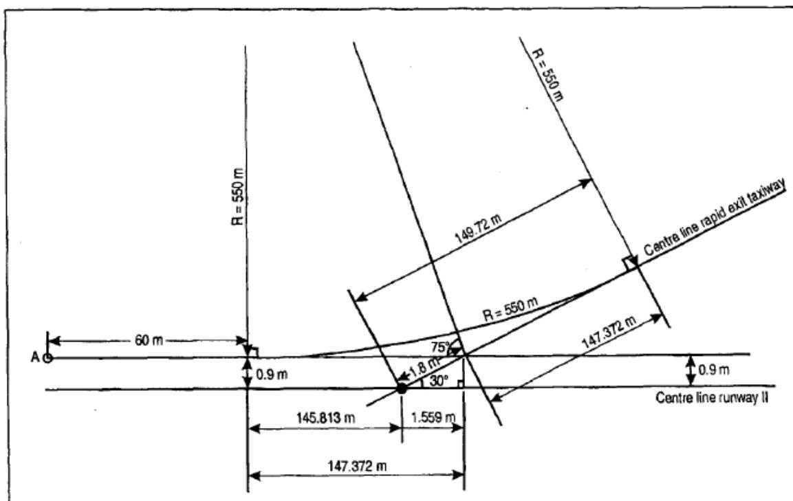
Below is an example of a rapid exit TWY design showing  $R$  figures of the curve design (not EKCH).
