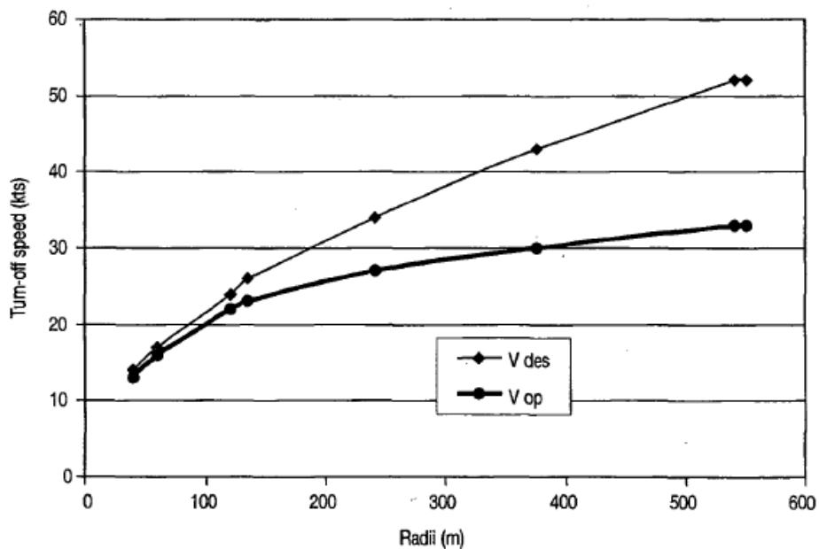
The graph is based on the design exit speed  $V_{des}$  complying with a lateral acceleration of 0.133 g, the operational turn-off speed  $V_{op}$  is determined empirically to serve as the criterion for the optimal location of the exit.
