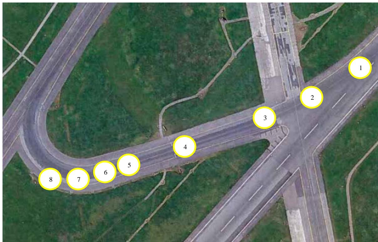
From the ACMS data it could also be revealed that the CMD deselected both thrust levers when the aircraft reached 60 knots GS. The reversers went to the FWD IDLE position before the aircraft reached the turn-off curve of TWY B4.
