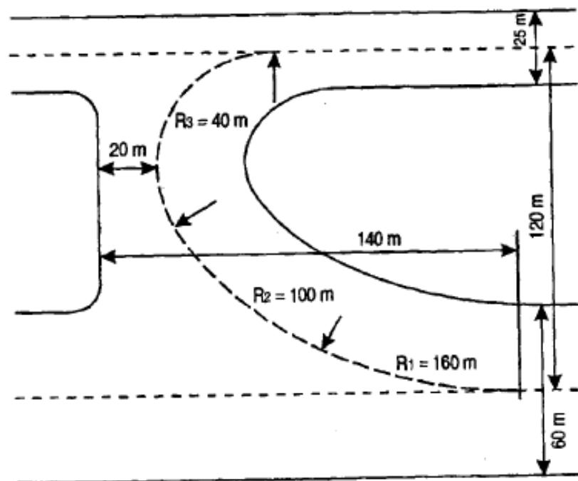
Taxiway curves should be compatible with the maneuvering capability and normal taxi speed of the aircraft for which the taxiway is intended.
