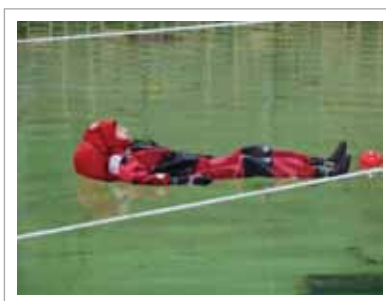
Subject during testing in calm water in pool at NRC–IOT (Exhibit 00221) ▶
