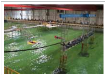
▲ Human performance and manikin testing in the testing pool of National Research Council – Institute of Ocean Technology (NRC–IOT) (Exhibit 00221)
