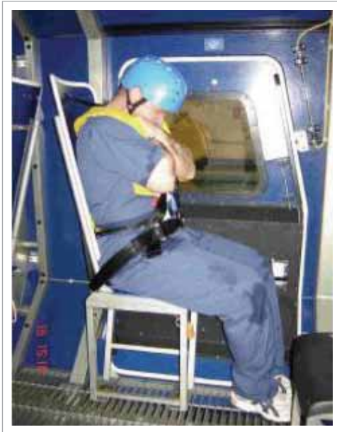
◀ High-back seat and four-point harness in HUET with trainee in brace position (Exhibit 00214)
