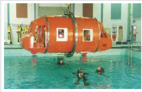
▲ Helicopter Underwater Escape Trainer (HUET) during survival training at the Offshore Safety and Survival Centre (OSSC), Marine Institute, Memorial University, NL (Exhibit 00018)
