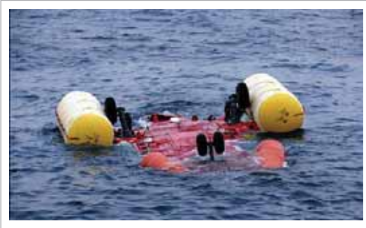
◀ Yellow floats deployed on inverted helicopter
