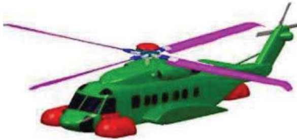
▲ Diagram depicting flotation equipment on S-92A in 2009 (Exhibit 00155)
