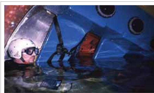
◀ Air pocket in interior of HUET with side flotation
