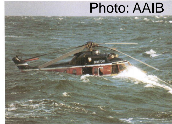
Bristow Helicopter registration G-TIGK, ditched (and later sank) after a triggered lightning strike in the East Shetland Basin; 19 January 1995
