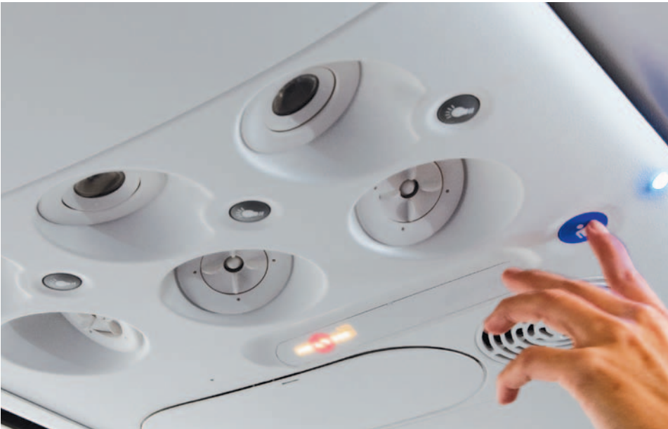
Figure 5: Passenger service units with integrated speakers
