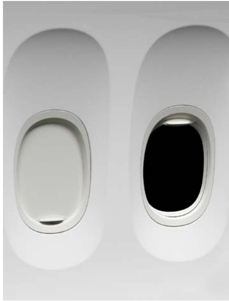
Figure 2: New cove lighting and window reveals
