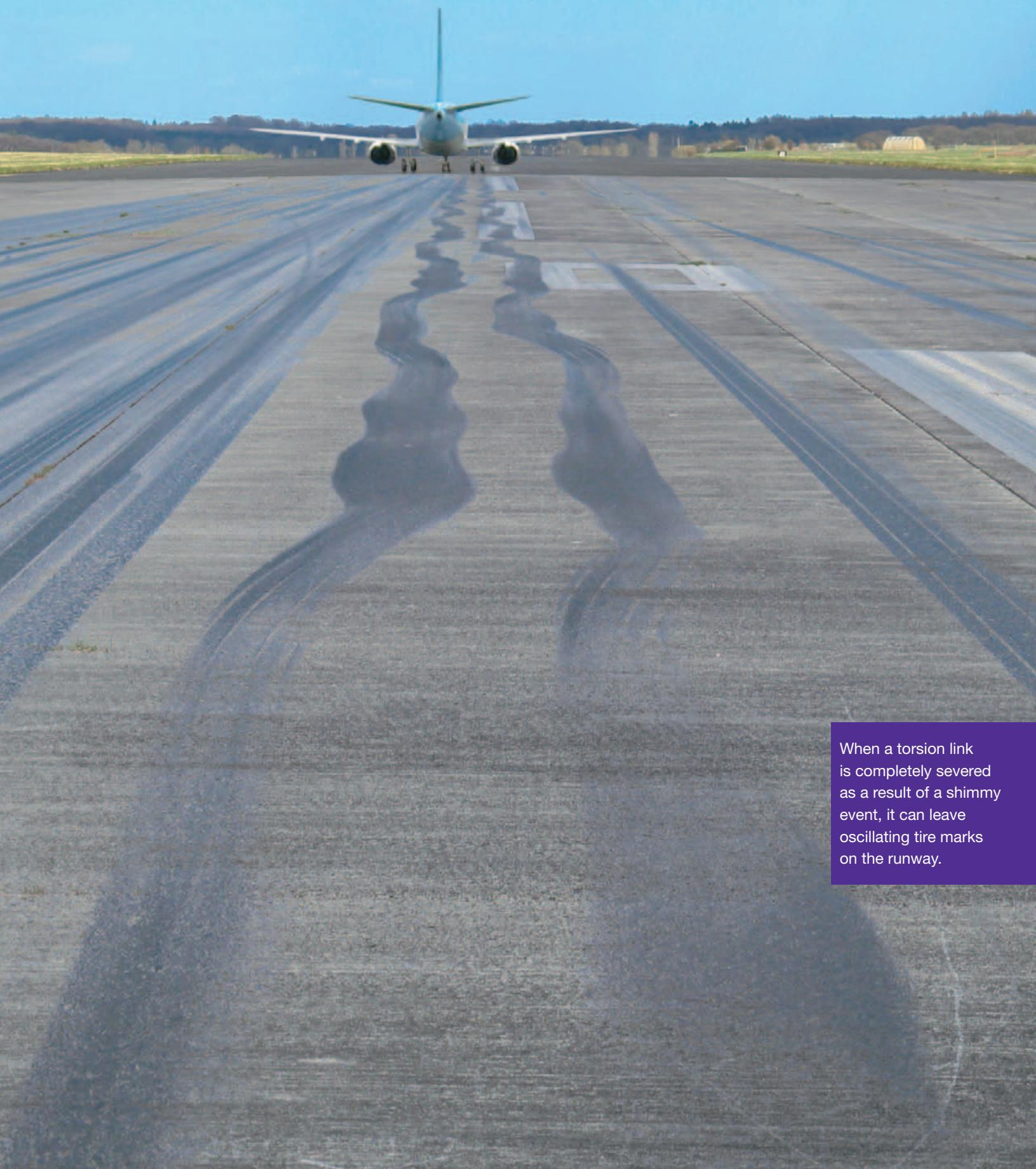
When a torsion link is completely severed as a result of a shimmy event, it can leave oscillating tire marks on the runway.
