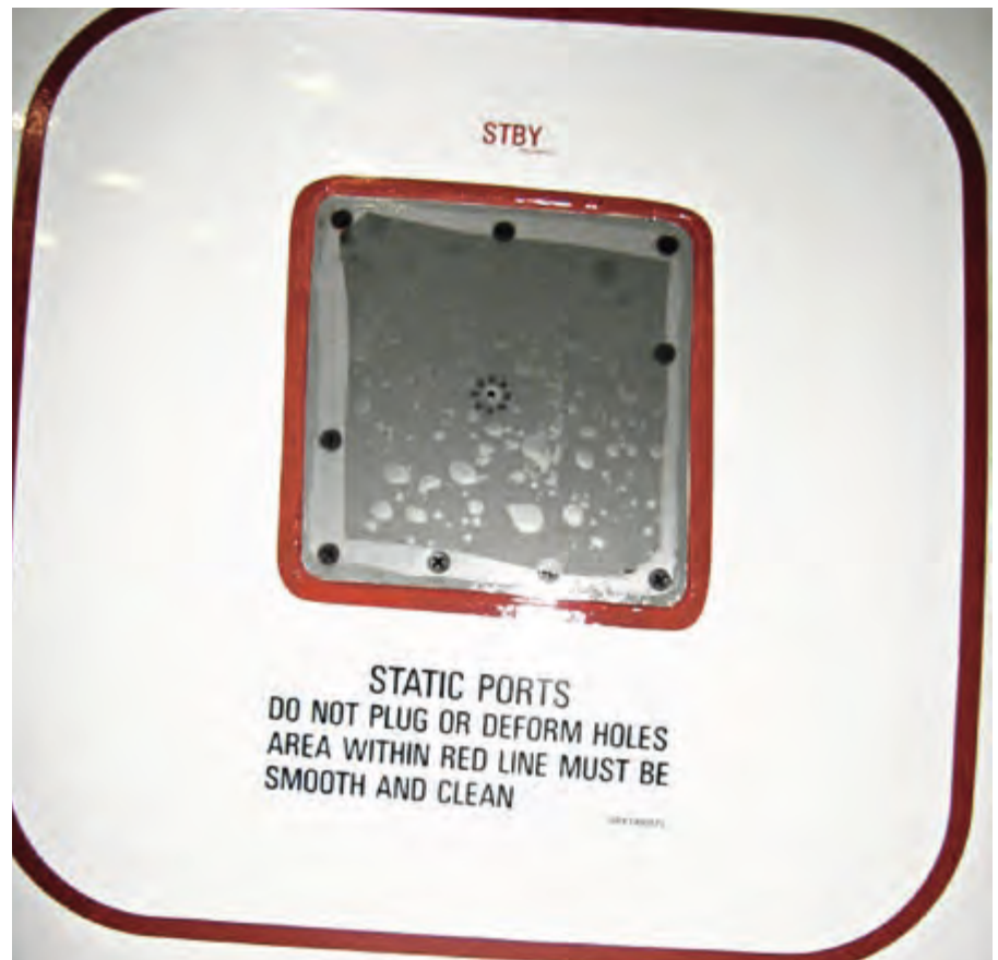
Figure 2 A clear plastic film over the static ports was left on the aircraft when it was handed back to the operator
