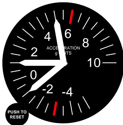
The Pitts S-2A is equipped with accelerometers (G meters) in both cockpits. These instruments measure acceleration parallel to the Normal axis of the aeroplane. That is to say the axis about which the aeroplane yaws. Sometimes this acceleration is called  $G_N$ , where the subscript 'N' stands for Normal.
