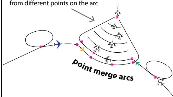
2. Aircraft fly the arcs until the aircraft in front is sufficiently ahead
