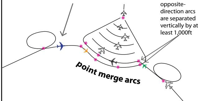
3. Aircraft are turned towards the merge point (A); aircraft are initially spread out as they fly from different points on the arc
