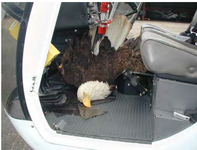
This helicopter was traveling at 80 MPH when it struck a bald eagle at 2,000 ft AGL. The eagle penetrated the windshield, striking a passenger in the chest. (Photo C. Cooper, Hummingbird Helicopters)
