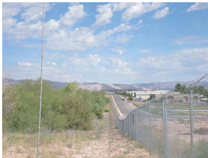
The FAA recommends a minimum 10-ft chain link fence with three strands of barbed wire for deer control. This type of fencing also greatly increases airside security. (Photo A. Dickey)
