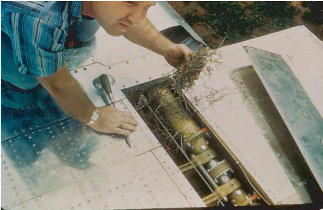
Collisions between wildlife and aircraft are not the only threat to aviation safety posed by wildlife. Here European starlings constructed a nest in the aircraft's wing. (Photo courtesy U.S. FWS)
