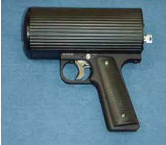
Under low light conditions, specially designed lasers can be effective in repelling geese, cormorants, and other birds. (Photo courtesy USDA)
