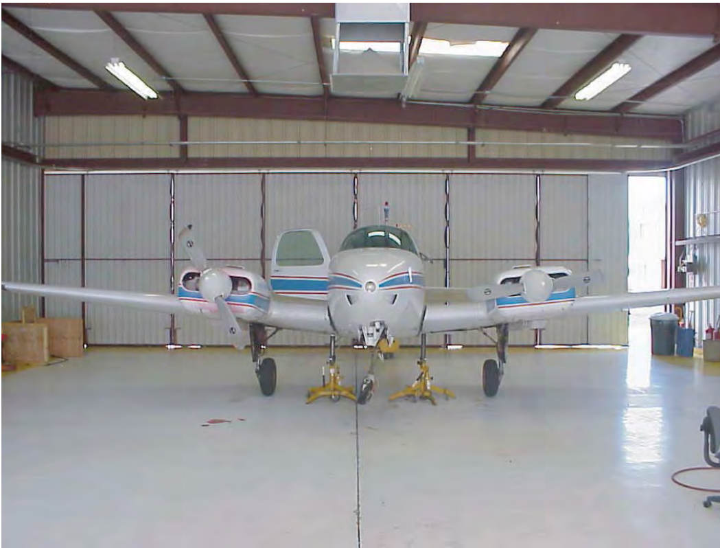
This Beachcraft Baron struck an 80 lb chow dog that ran in front of it during a night departure. The center landing gear collapsed and both propellers struck the ground. (Photo courtesy FAA)
