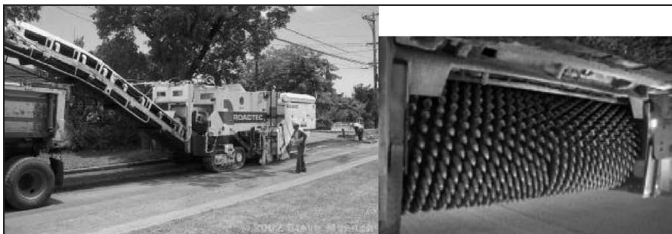
FIGURE C13 Milling machine and milling head (Washington 2002).
