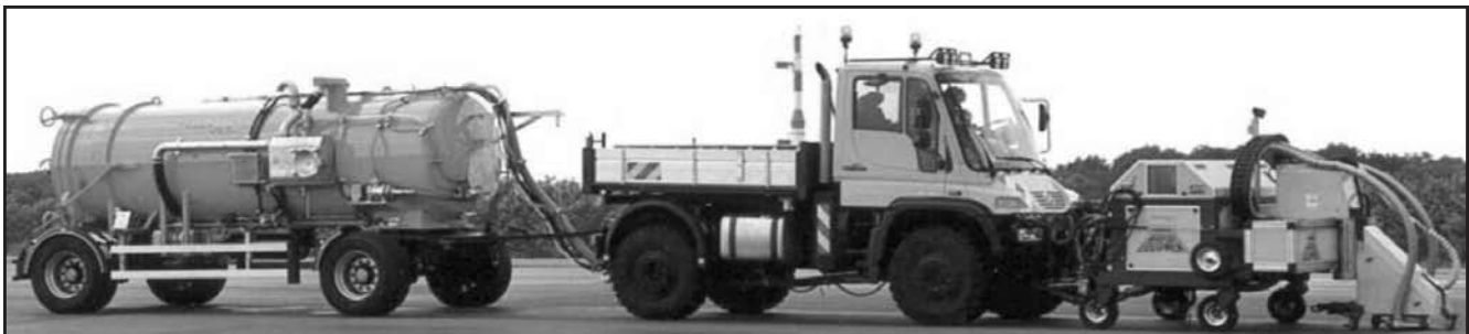
FIGURE C2 European vehicular-mounted and controlled waterblaster (Pade 2007).
