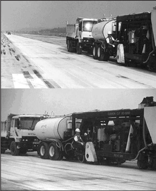
FIGURE C15 Diamond grinder in operation on airport (McLake 1999).
