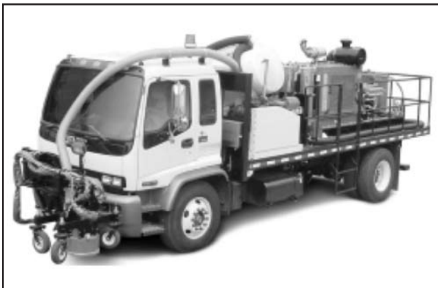
FIGURE C1 North American vehicular-mounted and controlled waterblaster (NLB 2007).
