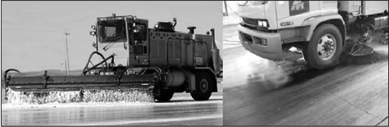
FIGURE C5 Vehicular-mounted and self-contained chemical distributor (Monkeman 2006; Saric 2006).
