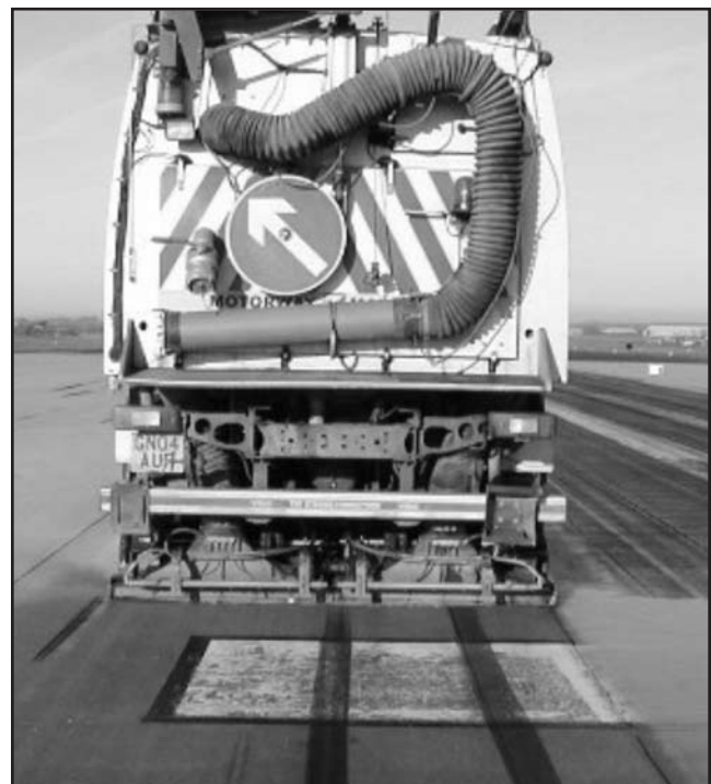
FIGURE C6 European vehicular-mounted chemical distributor (Zoorob 2001).
