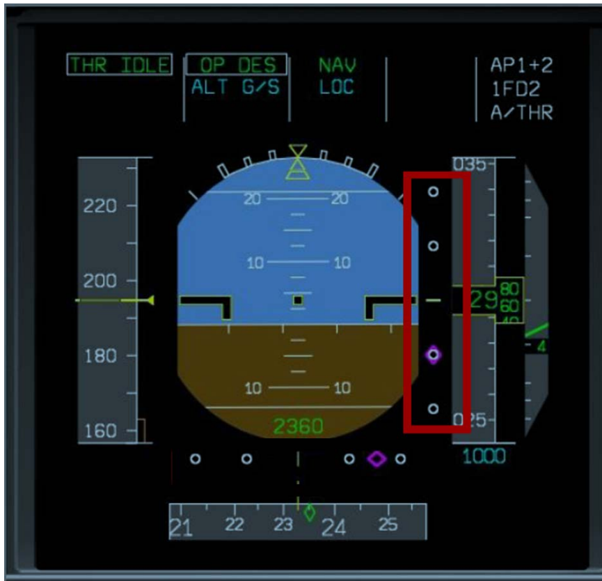
Figure 3: A330 primary flight display with the glide slope indication scale highlighted in red
