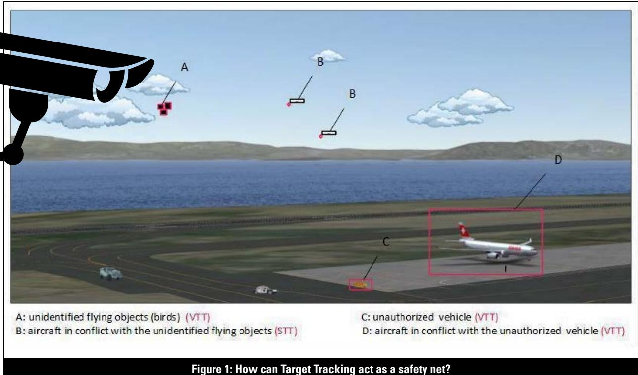
Figure 1: How can Target Tracking act as a safety net?
