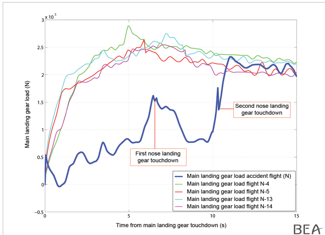
Figure 20: comparison of the vertical loads on the main landing gear
