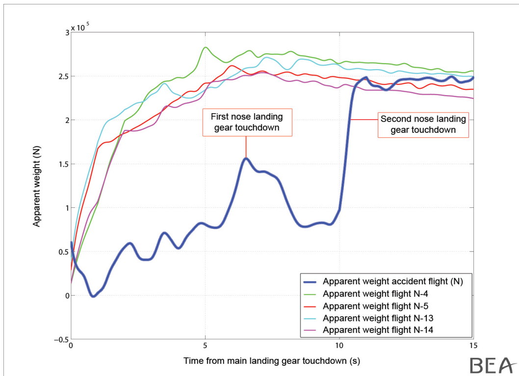
Figure 17: comparison of the apparent weight
