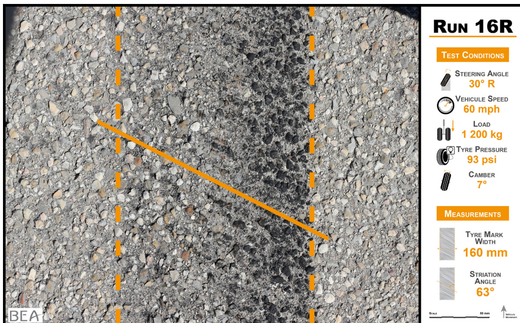
Figure 3: photograph taken at the end of a test
