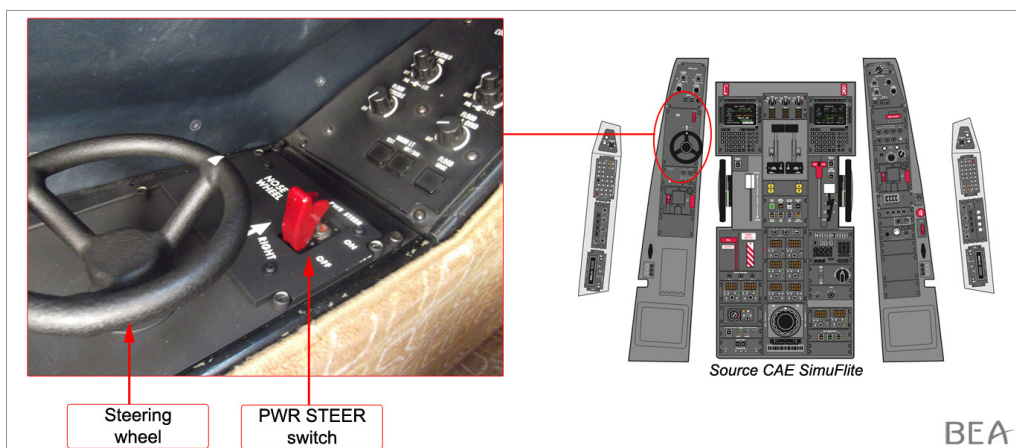
Figure 4: tiller and guarded PWR STEER switch
