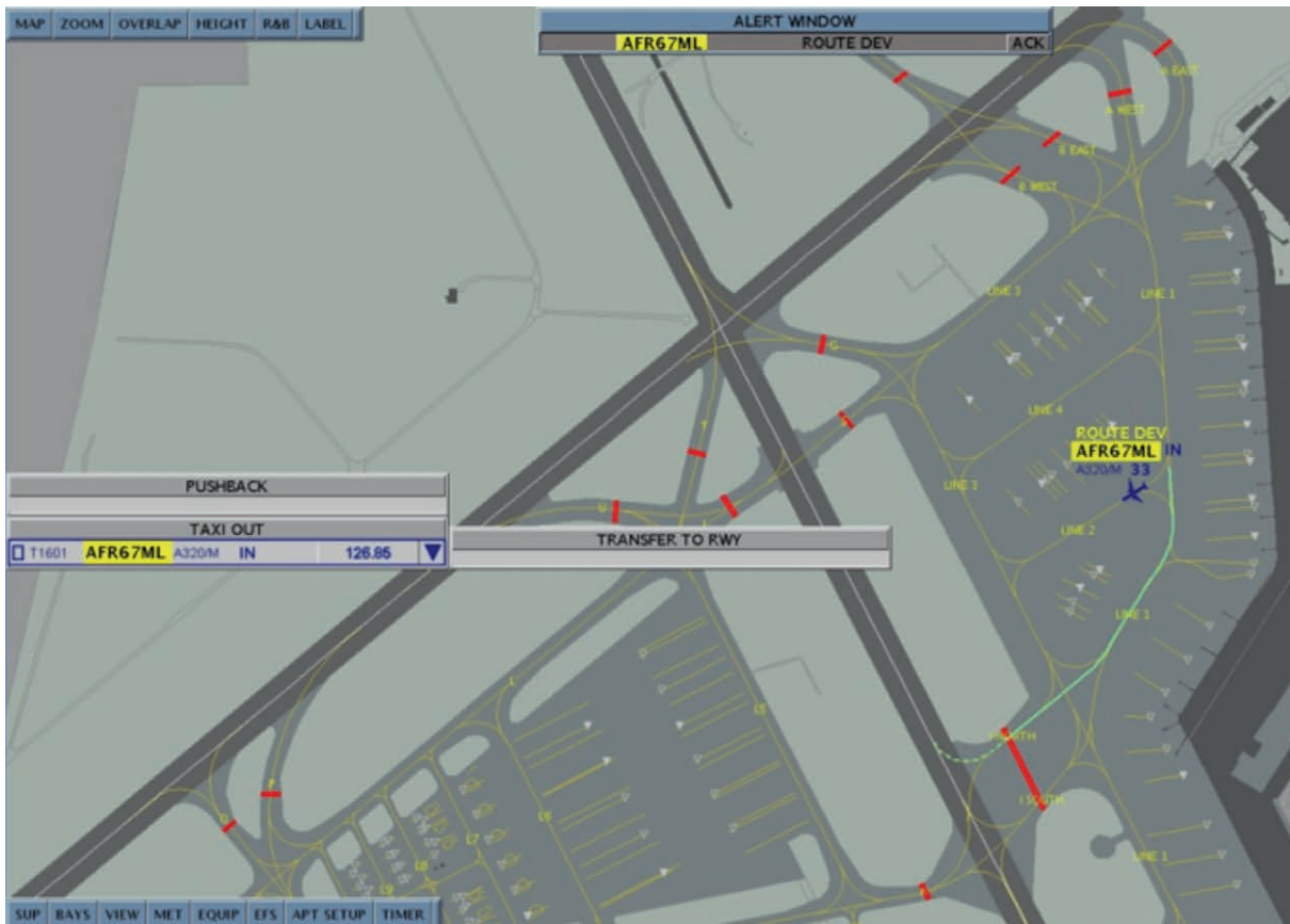
Figure 14. Yellow Highlight appears in Alert Window at top of display and yellow highlight on aircraft symbol and in Taxi bay for an aircraft that has deviated from the cleared routing.
