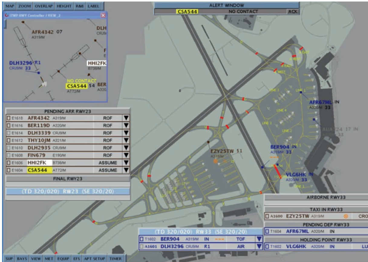
Figure 10. Yellow Highlight appears in Alert Window at top of display and yellow highlight on ATM element for no TWR frequency contact with an aircraft within 4 miles.
