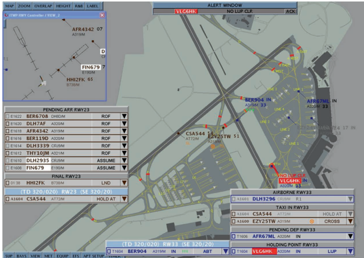
Figure 12. Red Highlight appears in Alert window at top of display and red highlight in Holding point bay and runway entry point for an aircraft that is entering the runway without a clearance.
