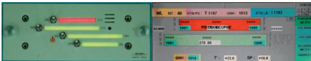
Figure 6. Picture to the left (above) depicts the Runway closed and to the right the associated ATC MET Report Display is depicted with wind information suppressed. NOTE, when the runway is occupied the light is blinking red.
