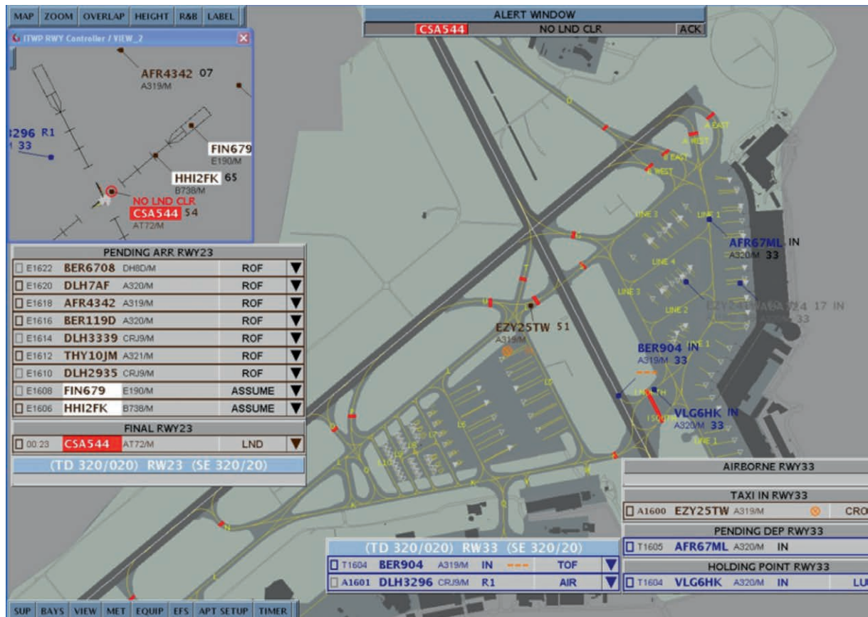
Figure 11. Red highlight appears in Alert Window at top of display and red highlight on ATM element and Arrivals elements for aircraft with no landing clearance within 1 mile.
