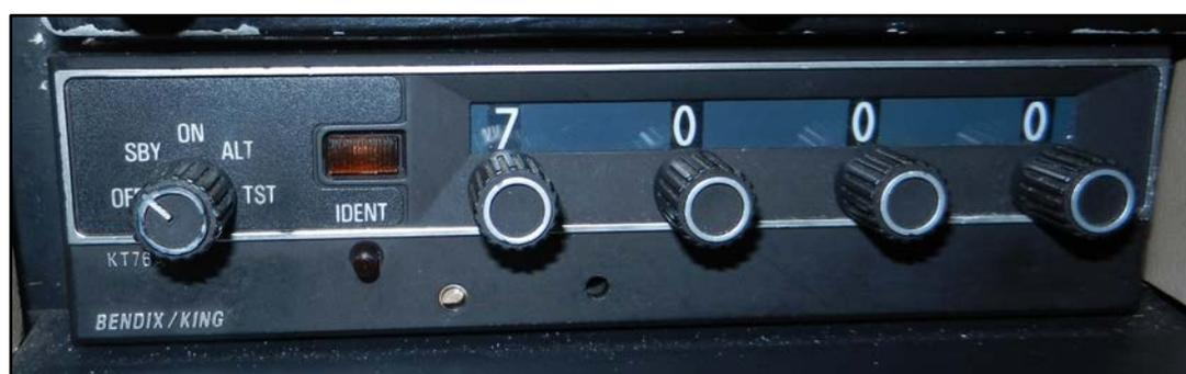
When the mode selector switch was set to “ON” (Mode A), the transponder code information was transmitted. If the mode selector switch was set to “ALT” (Mode C), the transponder transmitted both transponder code and aircraft altitude information.
