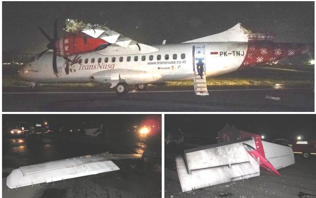
Figure 4: The detached part of wing and horizontal stabilizer
