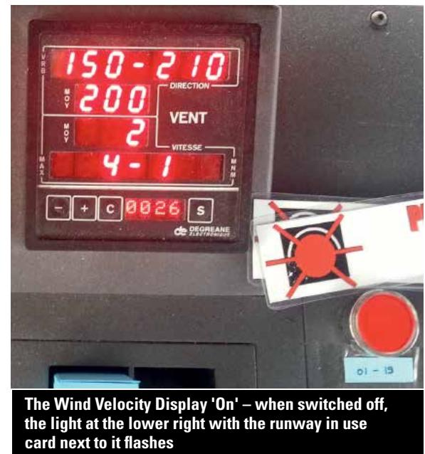
The Wind Velocity Display 'On' – when switched off, the light at the lower right with the runway in use card next to it flashes
