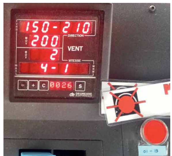
The Wind Velocity Display 'On' – when switched off, the light at the lower right with the runway in use card next to it flashes
