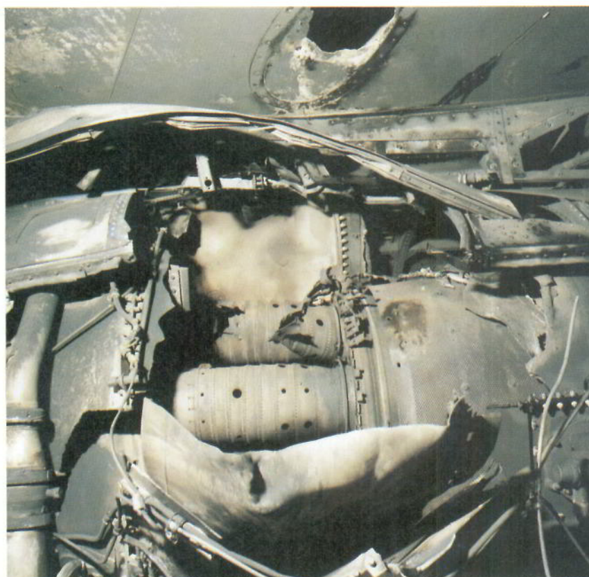
Engine rupture and holed fuel tank access panel
