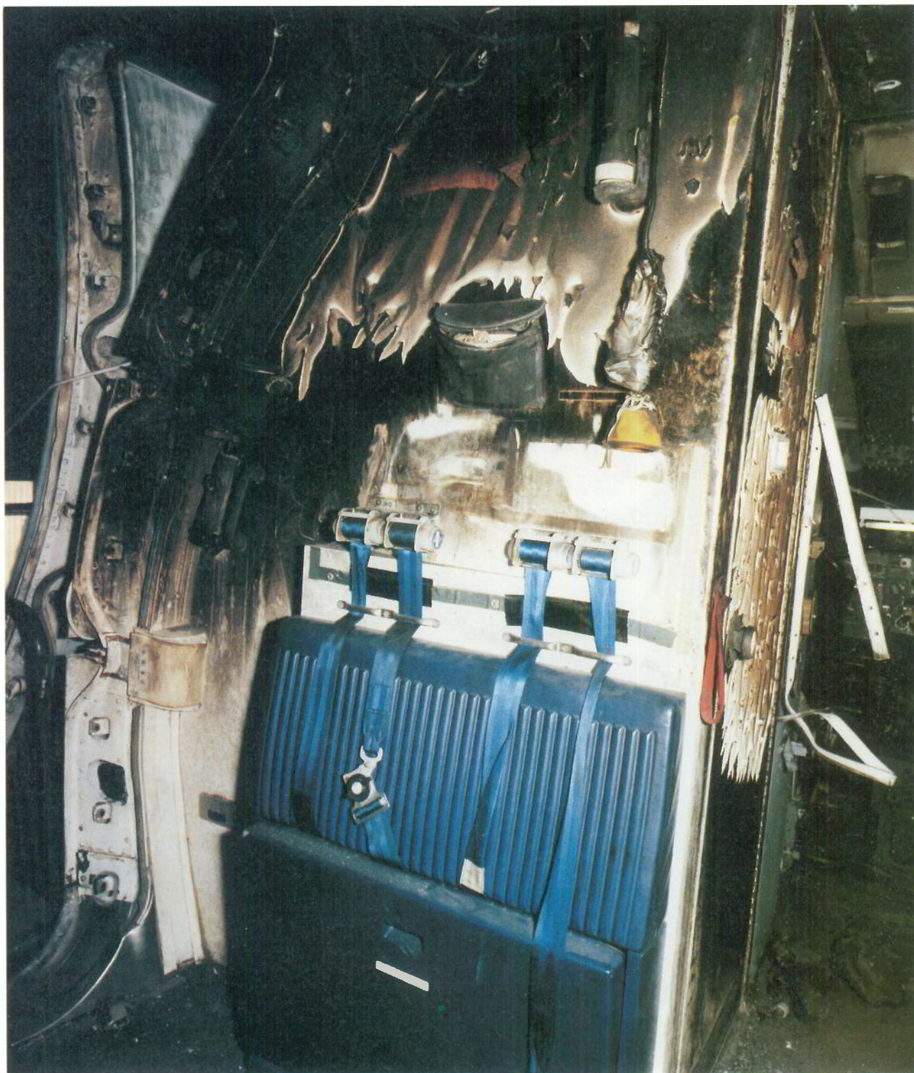
Temperature Stratification Effects in the Forward Galley
