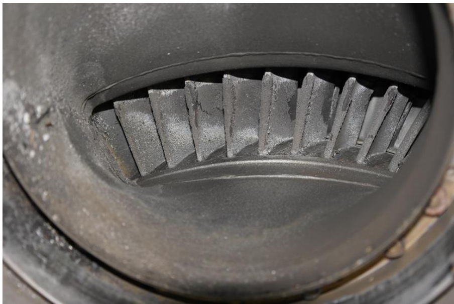
Figure 12: A section of HP guide vanes viewed through the nozzle box.
