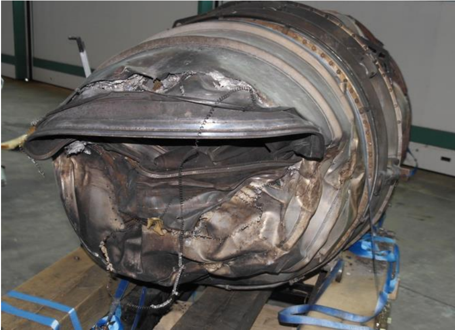
Figure 5: This is a view of the rear of the engine showing the distorted exhaust unit.
