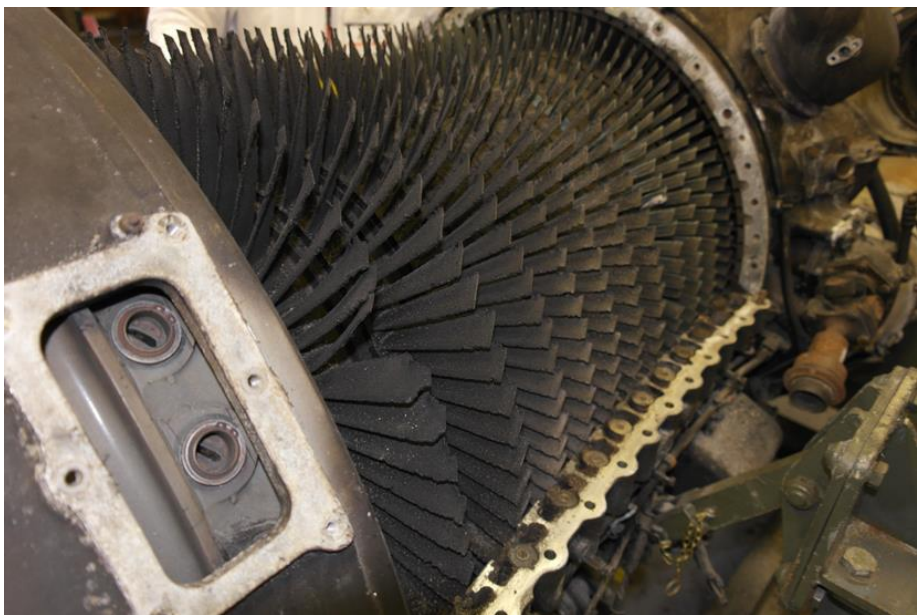
Figure 8: A general view of the compressor. Blade distress is clearly visible and the post-accident fire sooting is clearly visible.
