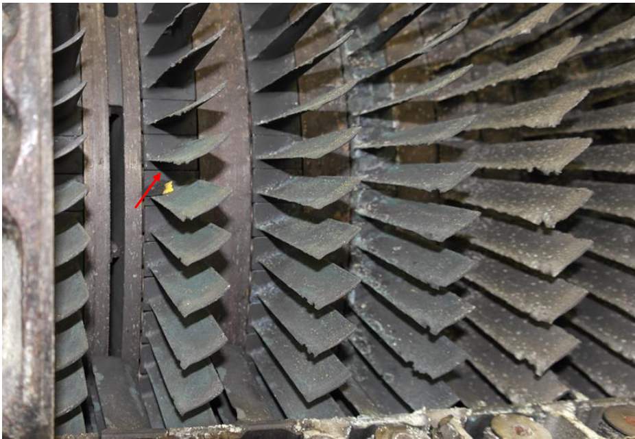
Figure 10: A piece of ingested debris was found within the stage 11 blades, (arrowed)
