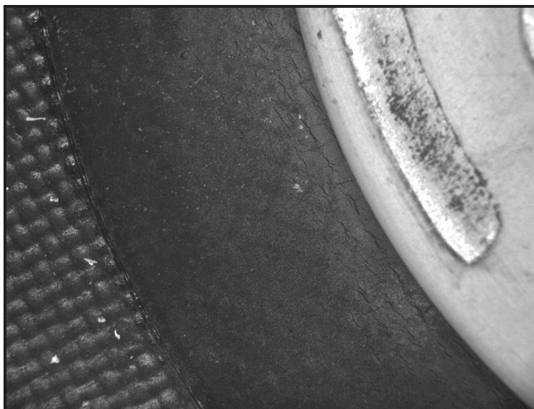
Figure 4 [REDACTED] GD64-1A Pump Diaphragm Cracking (Face 2)
