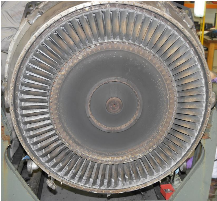
Figure 13: A general view of the 2nd stage (LP) turbine. All the blades were present and the general condition of the turbine was considered satisfactory.
