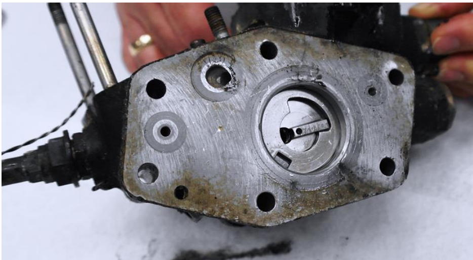
Figure 21: This is the opposite half of the shut off cock seen in figure 19. The valve was clean and its operation was smooth and unrestricted.
