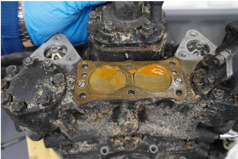
Figure 14: A general view of the dual fuel pump after removal of the fuel inlet cover. The orange coloured liquid is the result of post-accident water ingress.
