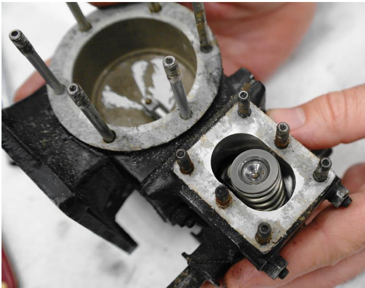
Figure 25: Another view showing the clean condition of the BPC adjustment housing.
