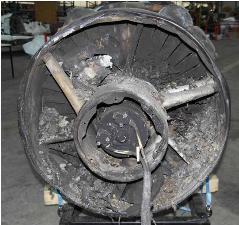
Figure 4: A view looking at the front of the engine. The level of ingested post-accident debris is clearly visible.
