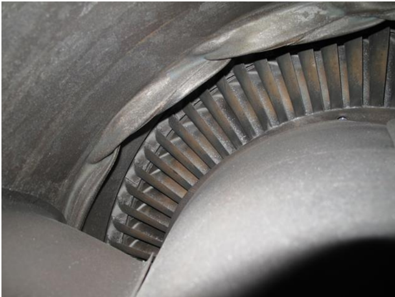
Figure 2: A section of the 2nd stage (LP) turbine viewed through the distorted exhaust unit.
