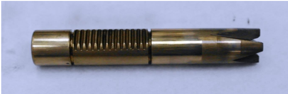
Figure 19: After removal of the metering plunger its general condition was considered to be satisfactory
