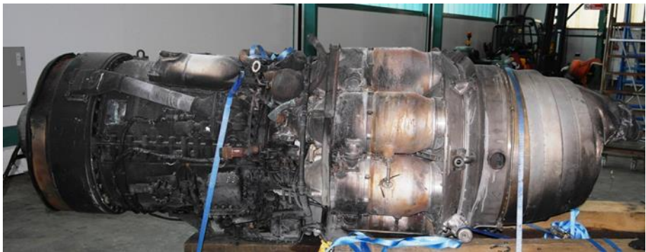
Figure 3: A view of the left side of the engine after removal from the airframe. Although the front half is coated in a layer of soot from the post-accident fire, the engine is complete.
