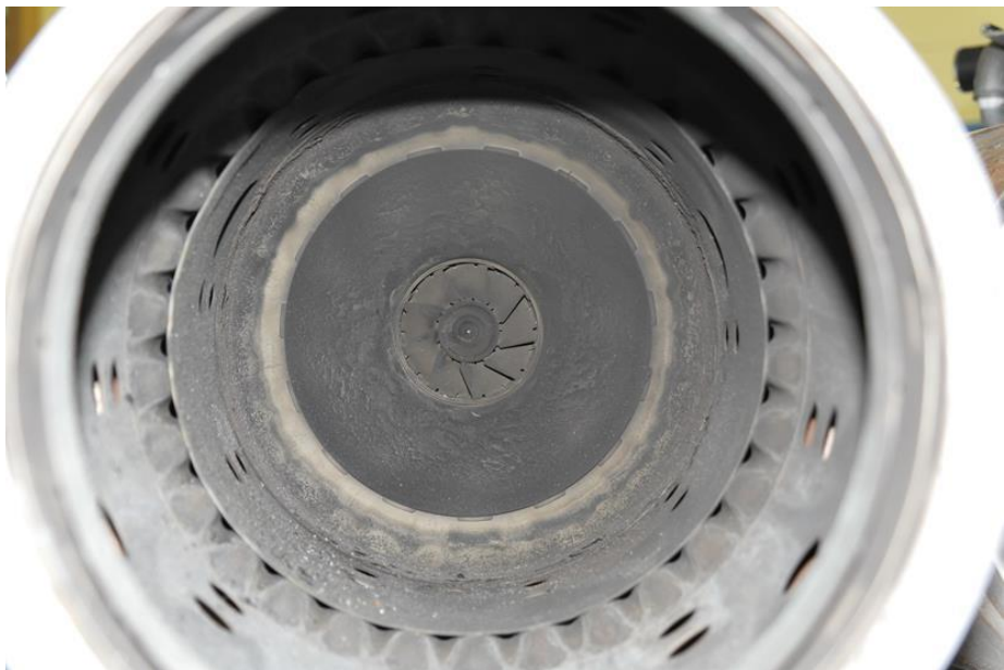
Figure 11: A general view inside one of the combustion chambers. All the inspected chambers were similar and considered satisfactory.
