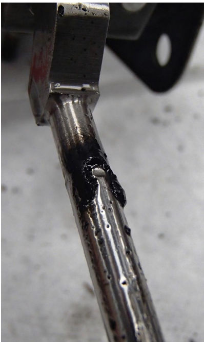
Figure 23: The pressure balance lever for the ACU which was considered to be in a good visual condition. The black deposit noted during the strip can be seen close to the needle roller contact point.
