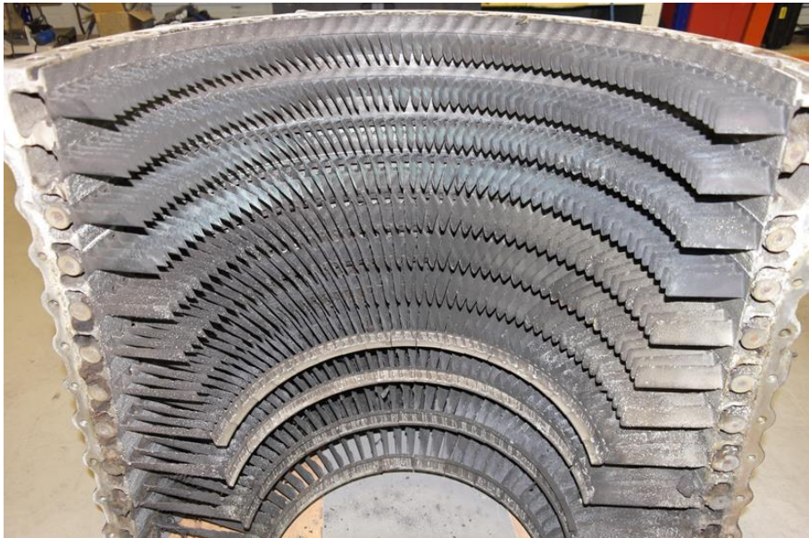
Figure 7: The top section of the compressor half casing. All the stator vanes are present but are coated in a layer of post-accident fire soot.
