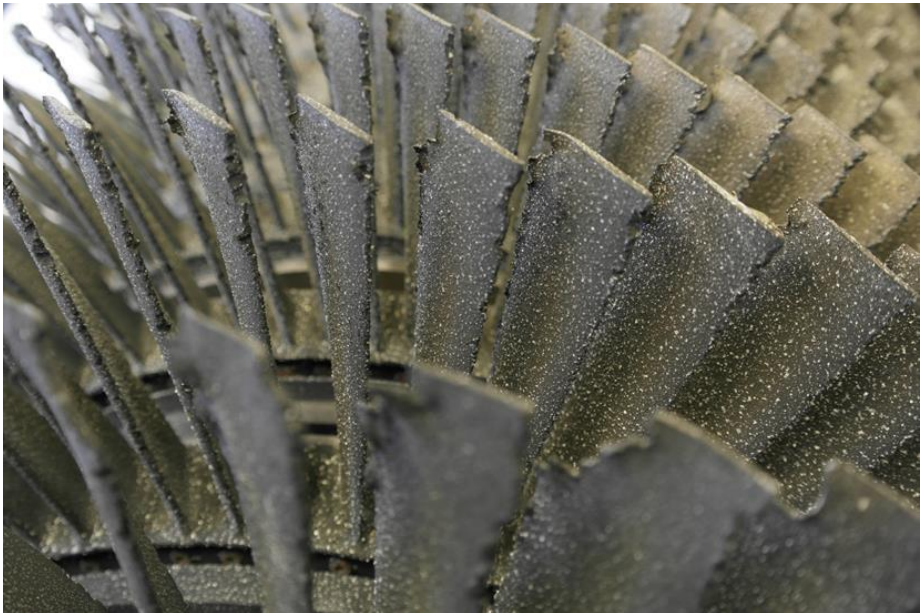
Figure 9: a close up view of the mid-stages of the compressor. Damage to the leading and trailing edges of all the blades can be seen.
