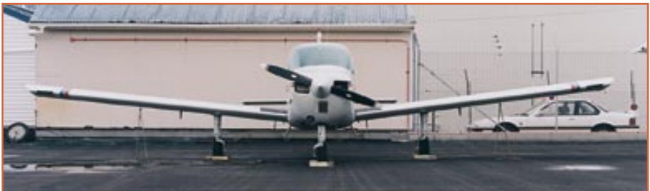
Picket your aircraft in a sheltered place – Seek local knowledge for the best place to secure the aircraft.
