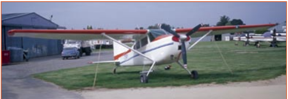
A tailwheel aircraft secured to fixed tiedowns anchors.
