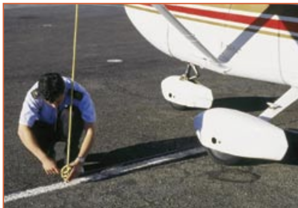
When tying ropes, draw them tight (not stretched) and then back them off a few centimetres.
