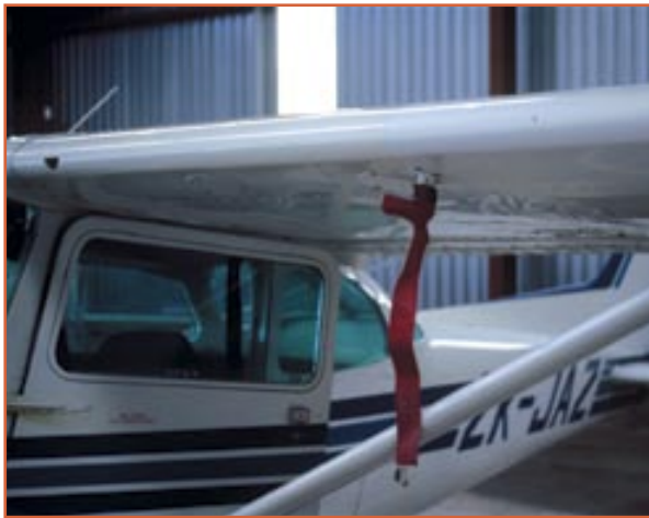
Pitot tubes should be covered to prevent the ingress of windblown dust and dirt. Remember to remove the cover before flight!
