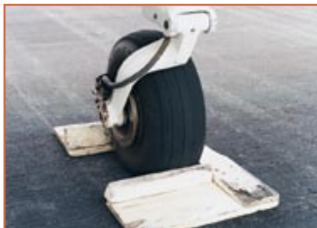
Chock the main wheels fore and aft.
