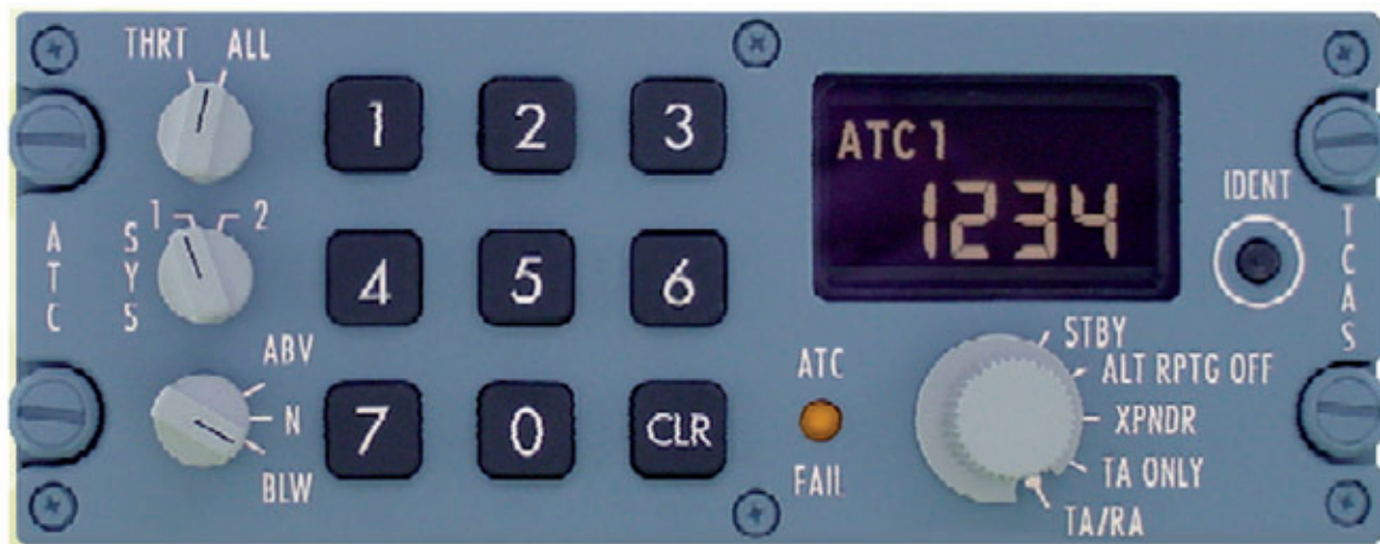
Fig 2: Gables 40 ATC/TCAS control panel
