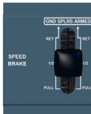
Figure 5 The ground spoilers were not armed
