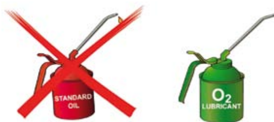
Figure 8 Use only oxygen systems approved lubricant
