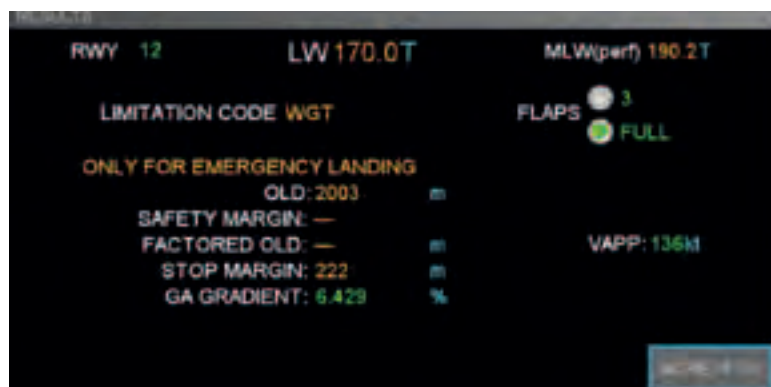
Figure 7 RWY COND: 2- Medium to poor FOLD longer than Landing Distance Available (LDA), but OLD less than LDA, results displayed in amber and MLW(perf) limited by OLD.
