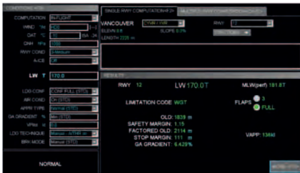
Figure 6 RWY COND: 3-Medium Runway not limiting, results displayed in green and MLW(perf) limited by FOLD
