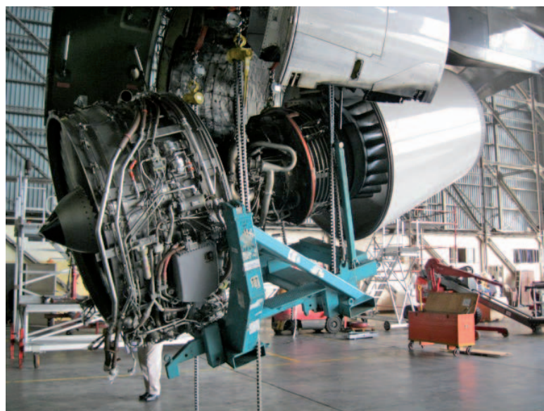
Figure 2 consequence of disengaged chain pulley
