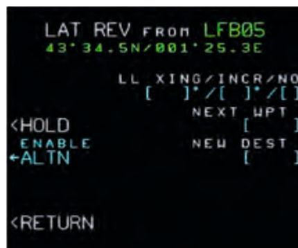
Figure 4 The missed approach remains available when discontinuing the approach. However, the FMS may have “lost” the destination
