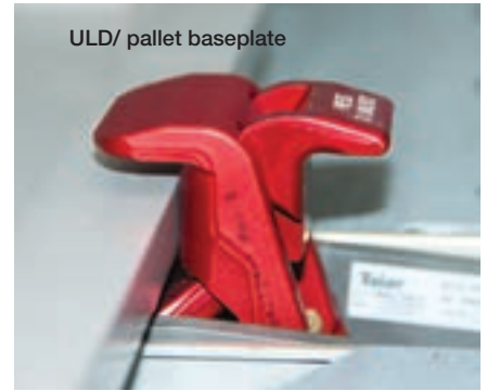
XZ latch raised and locked Interface with ULD/ pallet baseplate
