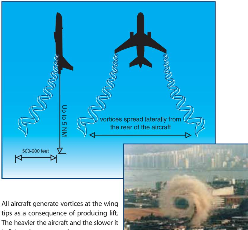
All aircraft generate vortices at the wing tips as a consequence of producing lift. The heavier the aircraft and the slower it is flying, the stronger the vortex.
