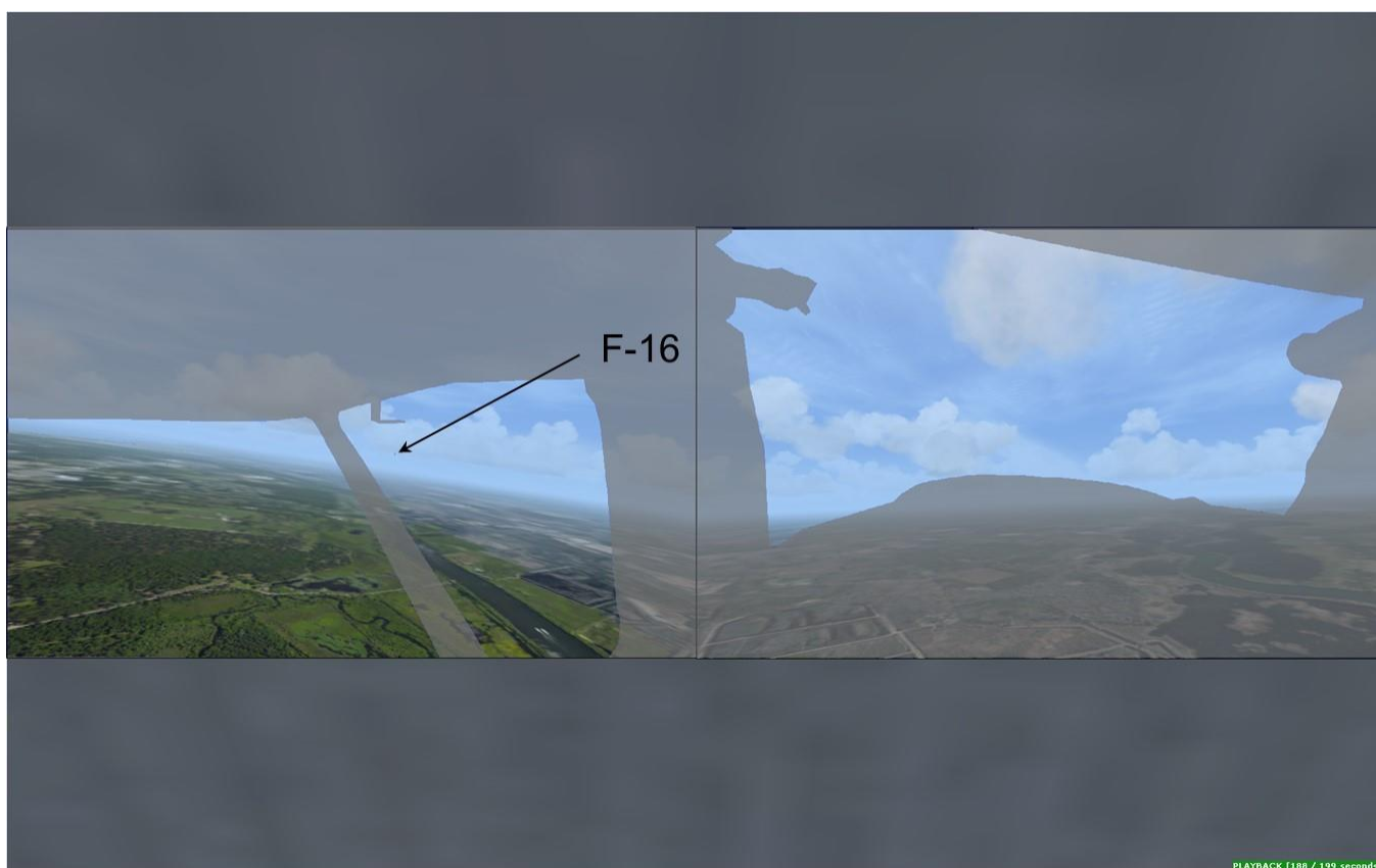
Figure 4b. Simulated cockpit visibility from the Cessna at 1100:49, when the airplanes were 0.6 nm apart.
