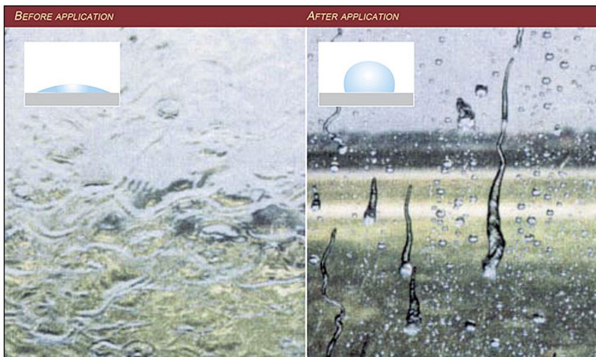
Figure 3. Illustration of the general effects of rain repellent at point of contact between drops of water and windshield. (Source: Airbus Industries Inc.)
