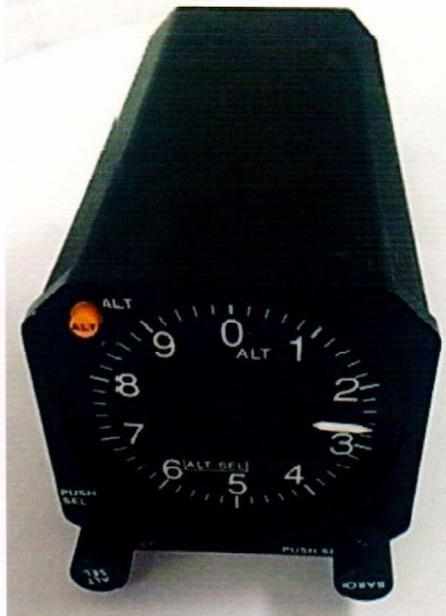
The Air Data Display Unit (ADDU) is a self-sensing, RVSM compliant, **digital air data computing (DADC) Altimeter** with selectable altitude alerting. The ADDU inputs static (Ps) and pitot (Pt) pressures, total temperature (Tt), and installation configuration data.
