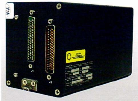
The Analog Interface Unit (AIU) is used in conjunction with the Air Data Display Unit (ADDU), **providing analog interface to the autopilot, navigation systems, and other using equipment.**
