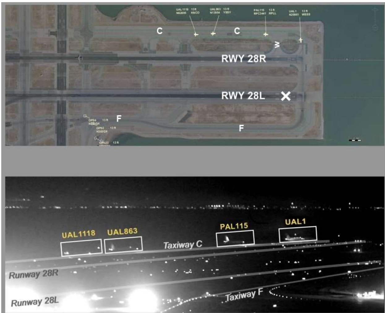
Figure 1 shows the positions of the airplanes on taxiway C. The top diagram is from Harris Symphony OpsVue radar track data analysis, and the bottom picture is from the SFO airport video. Altitudes are shown in mean sea level (msl); ground level is 13 ft msl. Airplanes in the top diagram are not to scale.
