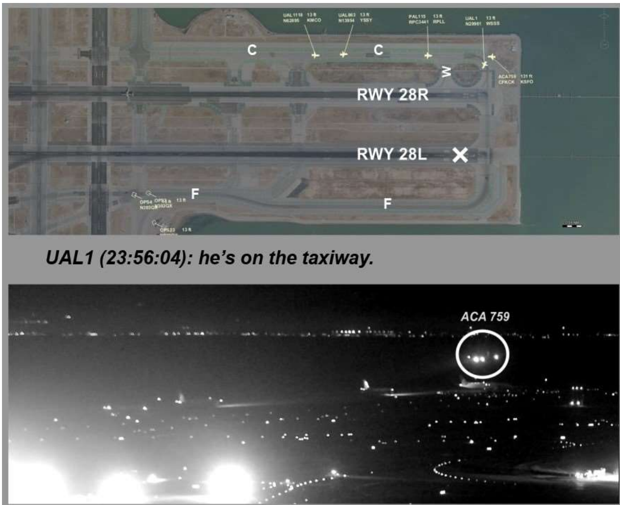
Figure 3 shows UAL1's transmission at 2356:04 and ACA759's position as it overflies the first airplane waiting on the taxiway; note that the second airplane has turned on its landing lights.
