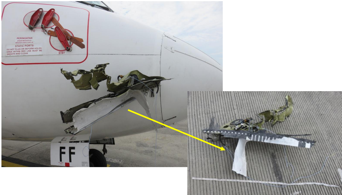
Figure 10: Part of the damage wing that stuck at the pitot tube
