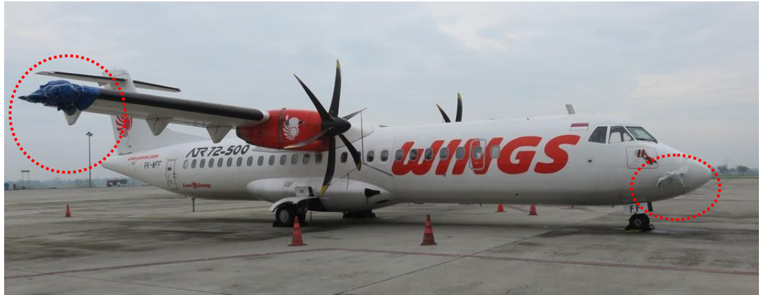
Figure 8: Damages on the right wing and part of wing that stuck at the pitot tube
