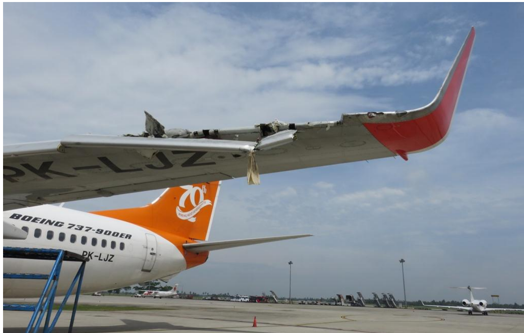
Figure 4: The damaged wing of JT197
