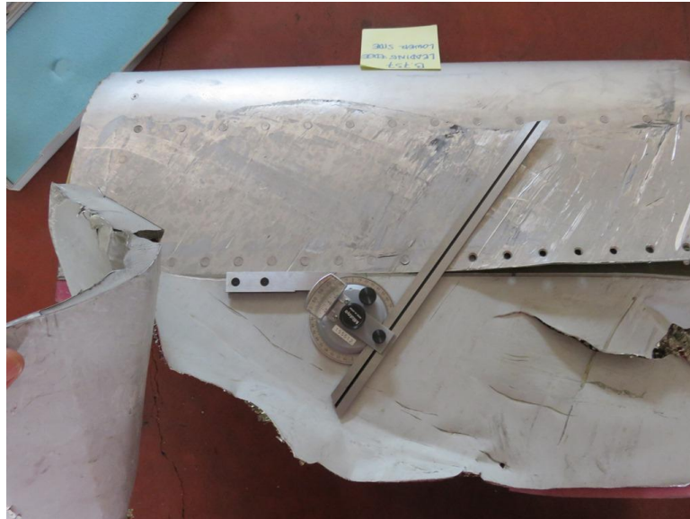
Figure 6: Part of slat number 1 recovered from the runway
