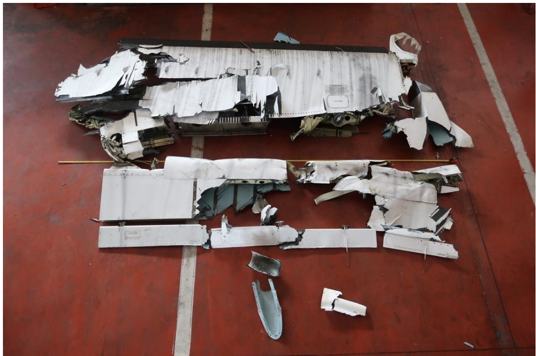
Figure 11: The reassembled wing
