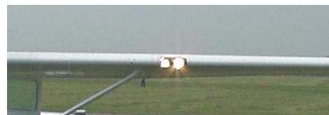
**Your aircraft lights** can help avoid collisions. High-intensity strobe lights, which can be installed at relatively low cost, increase your contrast and conspicuity a certain amount by day and even more by night. In areas of high traffic density, strobe lights are often the first indication another pilot receives of your presence. Consider the use of landing lights, especially in the traffic pattern and on hazy days.
