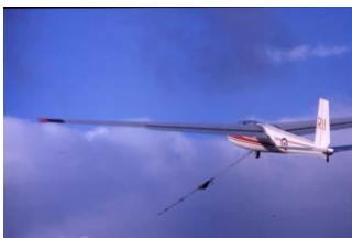
The area around a glider launching site is also likely to be very busy, apart from the hazard of colliding with a launch cable up to its notified maximum height. Aeroplanes towing gliders are less manoeuvrable than individual aircraft.
