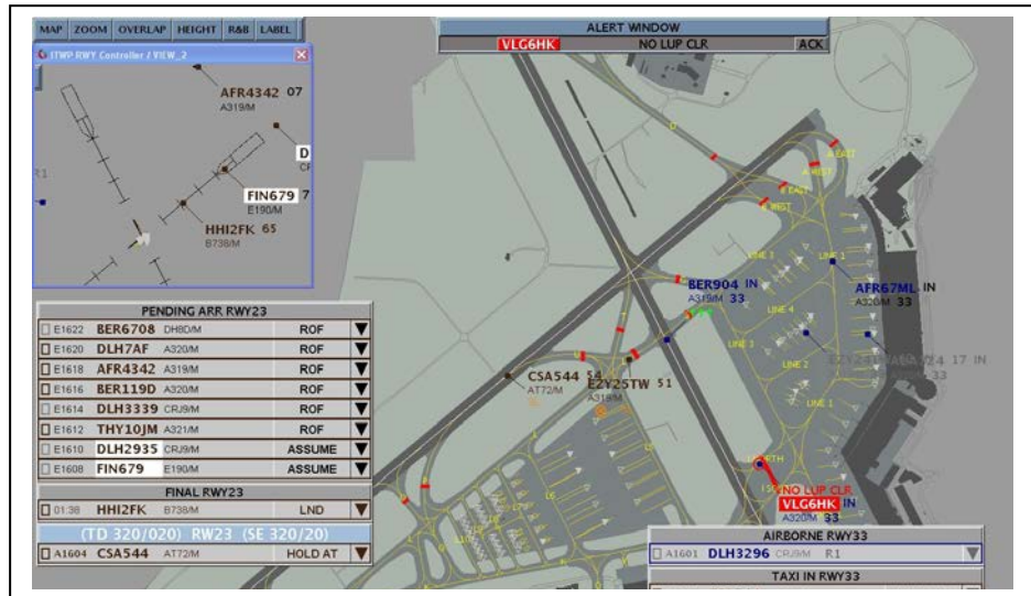
Fig 11. Red Highlight appears in Alert window at top of display and red highlight in Holding point bay and runway entry point for an aircraft that is entering the runway without a clearance.
