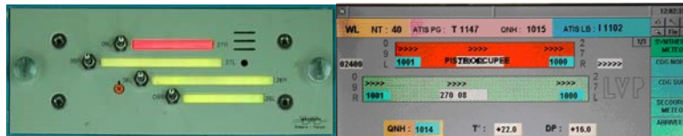
Figure 5. Picture to the left (above) depicts the Runway closed and to the right the associated ATC MET Report Display is depicted with wind information suppressed. NOTE, when the runway is occupied the light is blinking red.
