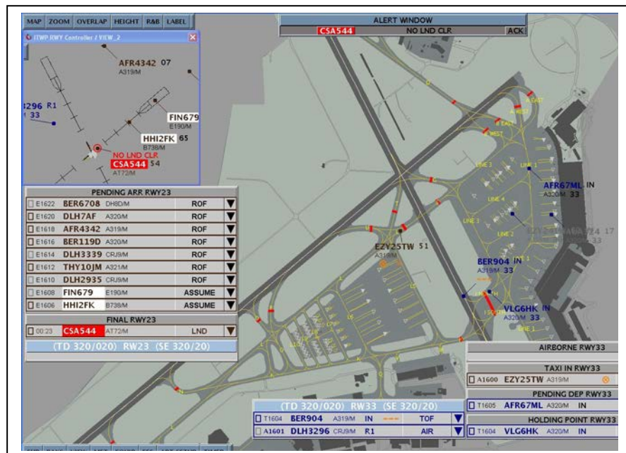
Fig 10. Red highlight appears in Alert Window at top of display and red highlight on ATM element and Arrivals elements for aircraft with no landing clearance within 1 mile.
