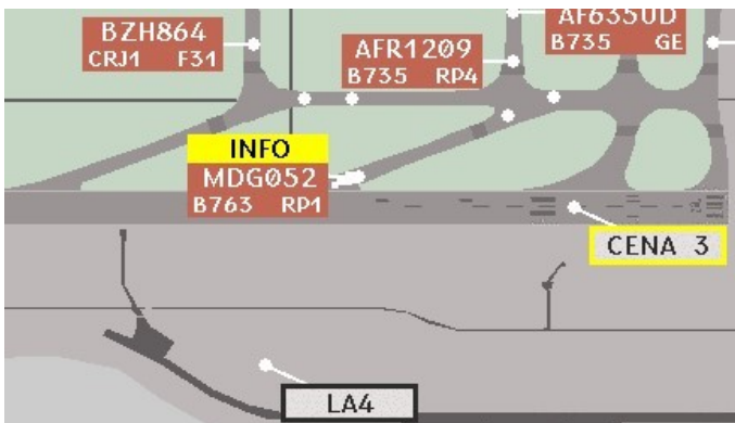
Figure 6. A-SMGCS display when an aircraft is in the runway strip and a car is on the runway.
