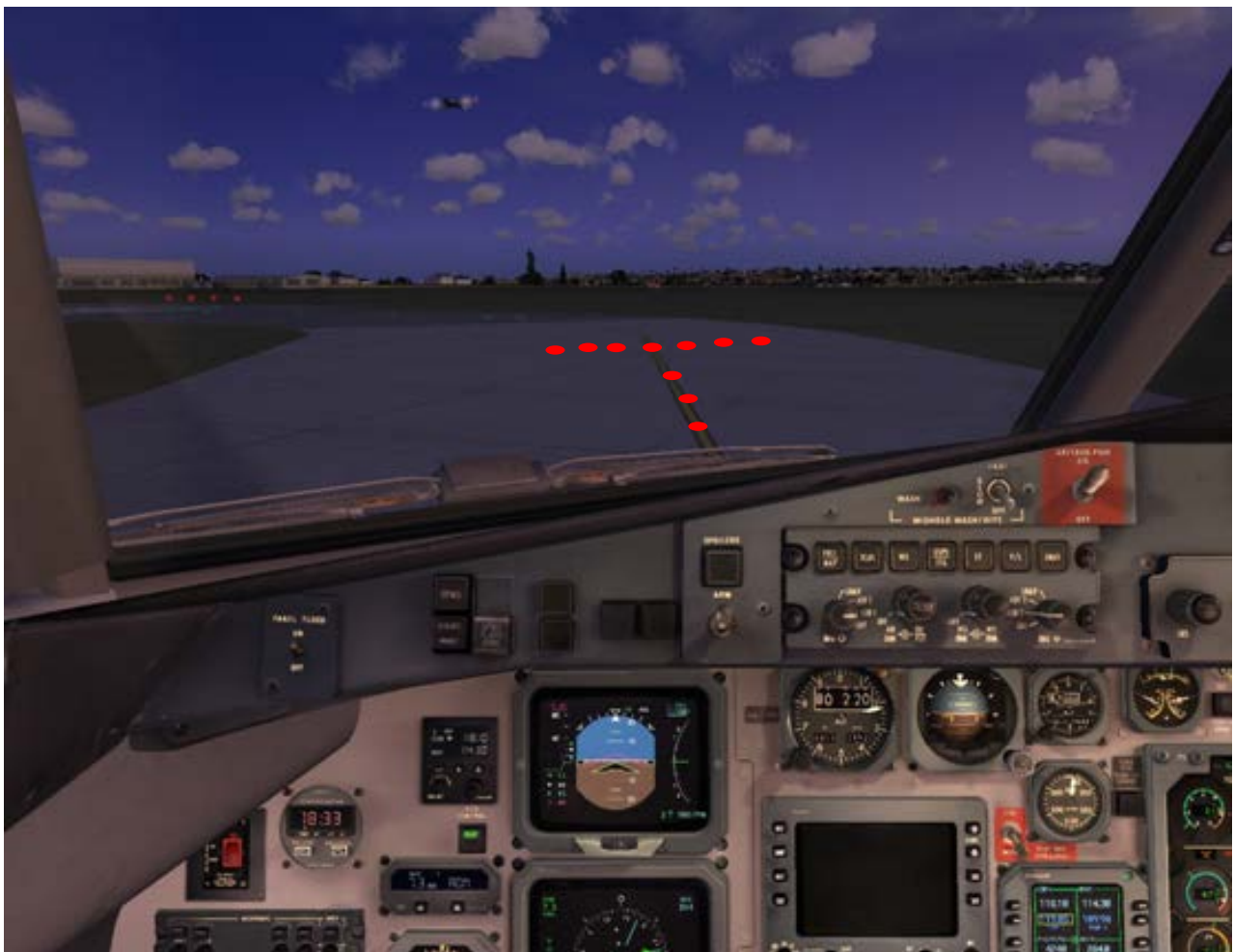
Fig. 19 Pilot view of SCIPS alert. Crossing an illuminated stop-bar results in array of Red Lights. 5
