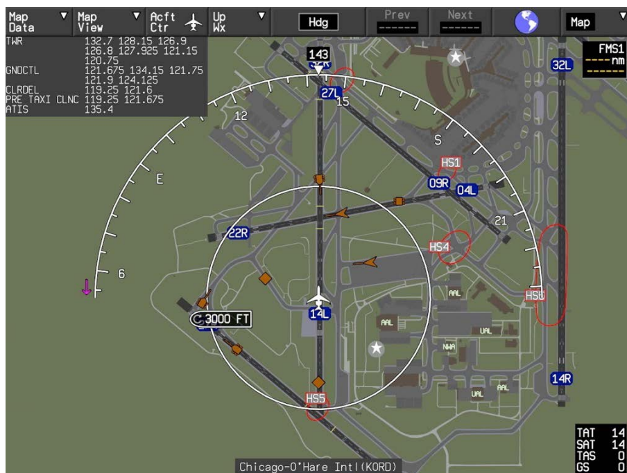
Fig 21 2D Airport Moving Map on Flight Deck Navigation Display 7
