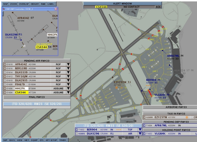
Fig 9. Yellow Highlight appears in Alert Window at top of display and yellow highlight on ATM element for no TWR frequency contact with an aircraft within 4 miles.
