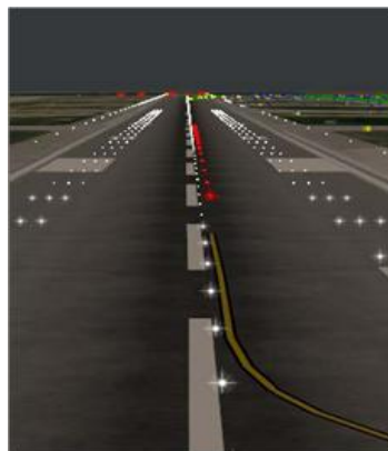
Fig.17 Pilot view of Take-off Hold Lights
